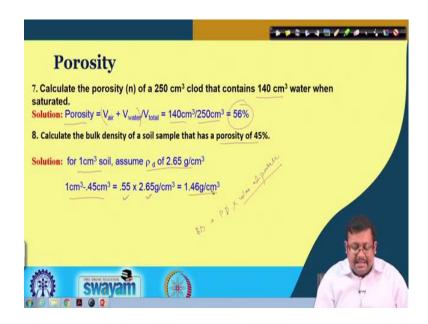
There is another question we know calculate the porosity of a 250 cubic centimeter clod that contents 140 cubic centimeter water when saturated.
