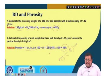
The number 5 fifth problem is calculate the oven dry weight of a 350 cubic centimeter soil sample with a bulk density of 1.42 gram per cc. Now we already know the bulk density is 1.42 gram per cc, we do not know the mass of soil; however, we know the volume of the soil that is 350 cubic centimeter.
