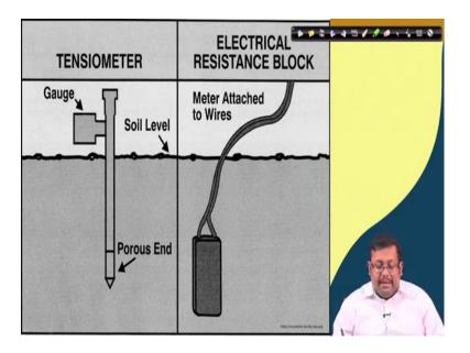
So, this is in a nutshell you can see the tensiometer, how these porous end is inserted into the soil and the gauge basically measures the vacuum and electrical resistance block where the meter is attached to the wires, which measures the electrical flow resistant to electrical flow based on the about the moisture which is absorbed.
