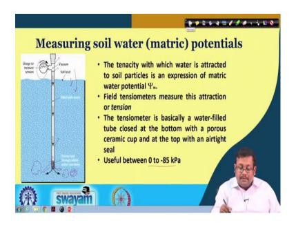
And another important instrument for measuring the soil water or I would say matric potential. So, it is called tensiometer or field tensiometers.
