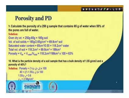
Now the last 2 questions are here calculate the porosity of a 250 gram of samples that contains 65 grams of water when 55 percent of the pores are filled with water So, you can see here the oven dry weight is give you know 250 gram minus 65 grams, so it is 185 grams of soil. Volume of soil solutes is the 185 gram over 2.65 gram per cc, so it is 69.8 cubic centimeter.
