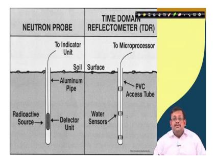
And this is neutron probe; we have already told that this is aluminium. You can see this is the aluminium access pipe and the, you know detector unit is inserted at the radioactive source is there and similarly time domain reflectometer or TDR, you can see there are water sensors and there is a PVC access tube.
