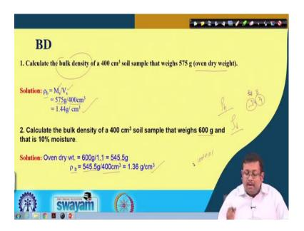
So, let us start with the bulk density calculation. So, you can see the first question is calculate the bulk density of a 400 cubic centimeter soil sample that weighs 575 grams which is it over dry weight.
