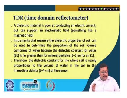
The another method is called TDR or type domain reflectometer. The time domain reflectometer works of the principle of time domain reflectometry. Now you know that a dielectric material is poor at conducting electrical current; however, it can support an electrostatic field something like a magnetic field and instruments basically the time domain reflectometer which you know which operates the principle of time domain reflectometery.
