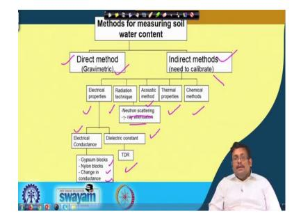
So, we have discuss about the energy concepts of soil. So, let us discus about different methods for measuring soil water content. So, we can broadly differentiate the methods of measuring soil water content into direct method and indirect method. So, direct method we will be discussing about the gravimetric, also we will be discussing about the volumetric method of soil water content.
