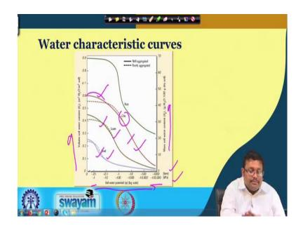
So, this curve is very much important, we call it water characteristic curve. So, in this water characteristic curve, it shows basically the relationship between the soil water potential and volume of soil water content or volumetric soil water content or gravimetric soil water content. So, we can see the x axis we are just plotting the soil water potential in log scale, remember that in log scale both in bars and kilo Pascal.
