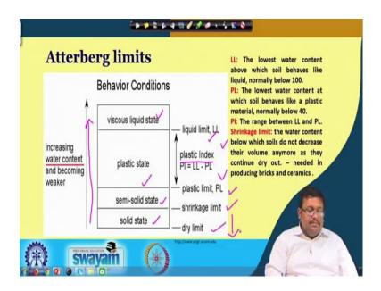
So, this is called Atterberg limits and in this Atterberg limits we can see we are seeing the plasticity be changing in the plasticity behavior of soil with increasing moisture content. So, you see that here you can you can see there are five different steps; five different stages or states I would say.
