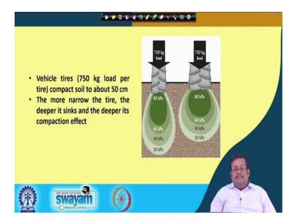
Obviously vehicle tires for example, 750 kg load per tires it is will compact soil to above 50 centimeter. And obviously, remember that the more narrow the tire the deeper it sinks and deeper its compaction effect.
