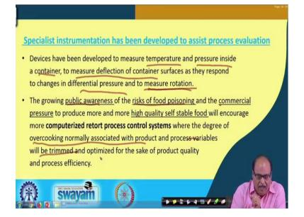
Special instruments have been developed to assist process evaluation, to measure temperature, and pressure inside a container, even to measure deflection of container surfaces as a response to changes in differential pressure, as well as even to measure the rotation of the container which is normally performed in order to improve the heat transfer efficiency.
