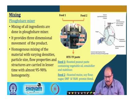
After that the next step is the mixing, in the ploughshare mixer you can see this is the picture. So, this as I showed you in the earlier flow diagram that there are two stream feed 1 and feed 3, feed 1 is the paste and feed 2 is the powder it is basically that is the solid and liquid mixing liquid or solid and paste mixing together. So, is the feed 1; feed 1 roasted peanut paste containing vegetable oil, emulsifier and stabilizers there.
