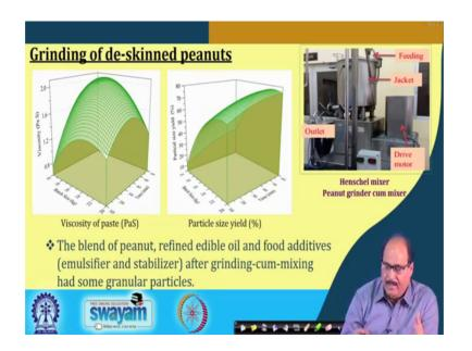
So, the this picture so that this is the picture of the Herschel mixture which is used for peanut grinding, cum mixing and this figure response surface graphs shows the effect of this time, temperature as well as batch size time of batch size and the viscosity of the peanut paste produced, as well as particle size that is particle size yield in the person particle size is are the peanut paste.
