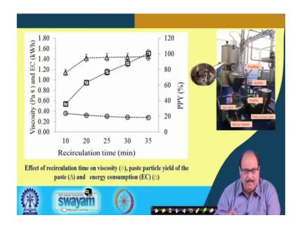
This consist this is the picture, so there is circulation time and then viscosity of the paste as you rise energy consumption and this paste particle yield. So, this is squares, these lines, this was the energy consumption, these your triangle points they show the paste particle yield and the circular points round points they show the viscosity.
