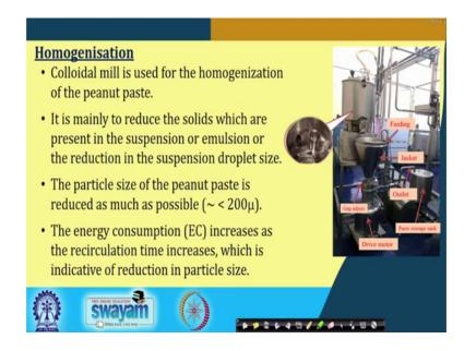
Then homogenizer, this is the picture of the actual or pilot scale unit, the material come it is a colloidal mill where the gas are properly adjusted rather to give the desired size particle size ok. So, finally, after the colloidal mill we get a homogenized paste material are of uniformly mixed material ok. So, in this basically this colloid mill reduces the solids which are present in the suspension or emulsion or the reduction in the suspension droplet size may be their.
