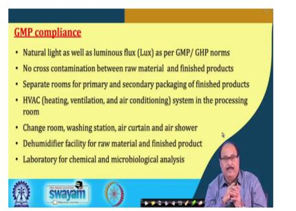
The GMP complaints is that is the plant is provided is to be provided for any plant which is GMP complaint here it should be provided for natural light as well as luminous flux as per the GMP GHP norms, that should not be any chance of any cross contamination between the raw material and finished products, the material handling some wind regulated in such a way. Similarly, there should be separate rooms for primary and secondary packaging of the finished ingredients.
