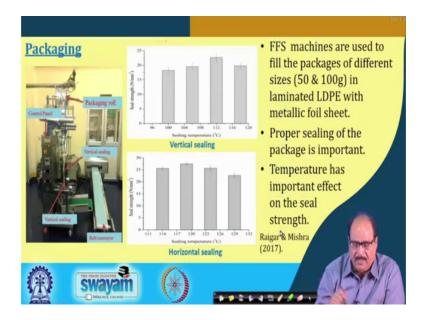
Packaging this is the form fill and seal machine which is used for the packaging of the size charts and in these packaging machines packets of starting from 50 gram to 100 gram or even more, having appropriate size and packaging machines. So, appropriate
