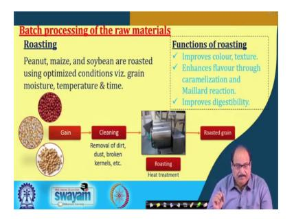
Then I will now with especially further those where in our piolet scale unit, these are the equipment pictures I am showing this we have a roster; roster which is a gives that thermostatically controlled and dry heating, we have the arrangement here where the temperature and time is set up properly can be maintained and even the temperature inside the grain, inside the roaster the grain temperature can be measured using this thermocouples or sensors.
