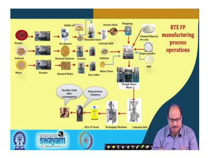
The same process you can see in this flowchart that is the ingredient wise, that is the ready to eat food paste manufacturing process operations that is three grains used is peanuts, soybean and maize. This is the passed through the roaster then de this peanut is de skinned, that is removal of the e skin red a skin.
