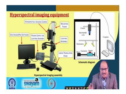
So, this the hyper spectral imaging equipment consists basically you can see here this is actual photograph of the hyper spectral imaging system which we have in our laboratory, so which has a schematic of this system is that it contains a camera that is the camera for taking the image which is right here, that is hyper spectral image in camera. And then some lighting assembly, lights are provided for illumination of the sample which is kept here.
