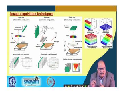
And this it is schematic representation of almost there that is there may be different types of image acquisition techniques like point scan, whisker broom configuration system there which use as a interferometer, the other case it is a line scan push broom configuration. There are dispersing filters and you can see there from the light source how the sample image is coming, and then data is sent to the dispersing filters, and finally it comes in the form of cubes.
