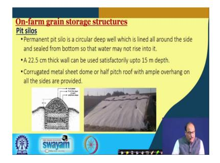
Then on farm storage structures include pit silos there is permanent pit silo is a circular deep well which is lined all around the side and sealed from the bottom so that water may not rise into it that is the soil water field water about 22 and half centimeter thick wall, is used and it becomes a satisfactorily 25 and half centimeter thick and it is it works satisfactorily up to 15 meter depth.
