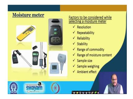
Similarly, the moisture meter there are different types of moisture meters are available in the market like NIR based moisture sensors, infra rate based moisture rate sensors and other sensing probes etcetera are available chemical method is available. So, depending upon that is whether chemical methods normally although they are provide good reliable data which is used commonly in the laboratory, but it is a time consume process.
