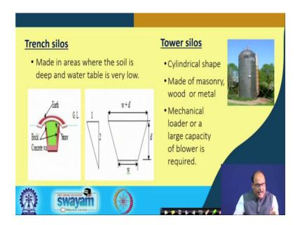
Corrugated metal steel dome or half pitch roof with ample overhang on the all sides may also be provided. So, you see here in this pit silos. The other are the trench silos which are made in the farm or the field it is the areas where the soil is deep and water table is generally low this trench silos are made. Tower silos they are cylinder in shape made of masonry wood or metal the mechanical ladder because they are very tall.
