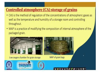
Then another important aspect is the controlled atmosphere, storage of grain as well we have already discussed in the earlier classes what the in the fruits and vegetables? What is the controlled atmosphere or how what is the modified atmosphere, but this can be applied as well to the grain you can see here that is low oxygen chamber of for the grain storage is shown in the figure.
