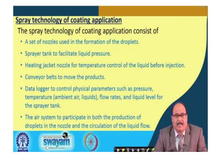
The other technology which is the most commonly used technology for the coating of the fruits, vegetables or many other food materials etcetera is the Spray technology. This spray technology for application of coating consists of a set of nozzles used in the formation of the droplet are used for the formation of the obviously, it has to be sprayed; so some arrangement for spraying of the coating solution over the surface of the food material ok.
