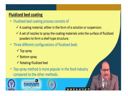
Another method is the Fluidized bed coating. Fluidized-bed coating process consists of obviously, a coating material. The solution of the coating and it may be either in the form of a solution or in the form of a suspension and then a set of nozzles to spray the coating material on to the surface of fluidized powder to form a cell type of structure.
