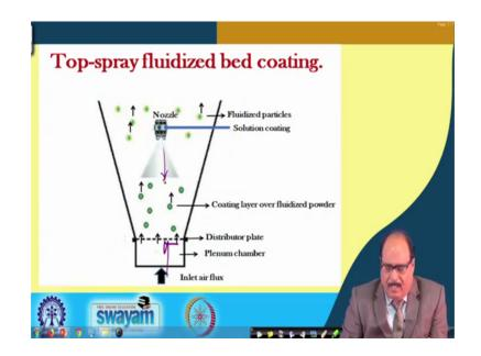
You see here that is a top spray fluidized-bed coating, the in this bed the inlet air flux. The material powdering material or fluidized powder, it gets fluidized and then the coating; coating solution is sprayed on the top through help of these nozzles and of course, this spray again there is the other arrangement which you have seen in the case of spray technology that.
