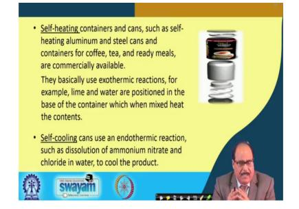
So, self heating containers and cans like for example, self-heating aluminium and steel cans and containers which are used for coffee, tea and ready meals etcetera. They are commercially available you can see in the picture here.
