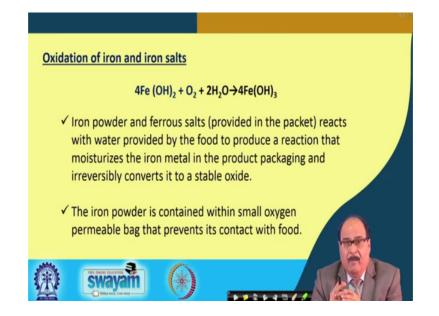
Here in this slide just I have shown you how the iron compound, the iron powder, how it oxidises right the ferrous salts or iron powders. They react with the water that is provided by the food to produce reaction that moisturizers the iron metal in the product packaging and irreversibly converts it to a stable oxide.
