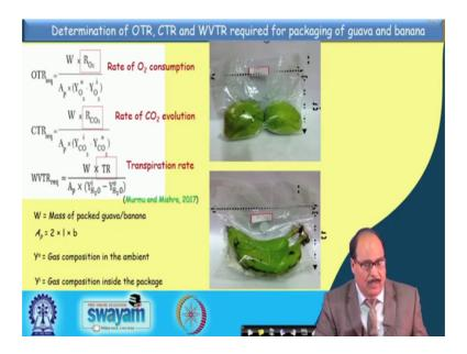
So, we have published this data that is we have given this model that rate of O 2 consumption rate of CO 2 evolution and transmission rate for the banana can be calculated that is using these equations that is OTR, CTR and WVTR are required for the packaging of guava and banana. All these we have provided these equations and data is available.
