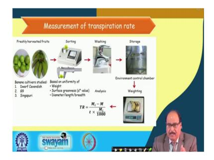
So, one can keep the material in the next slide. We will show you that transpiration rate how it they can be measured that is freshly harvested materials they can be put after of course, after sorting weighing etcetera. Then washed and it is packaged and kept into a suitable environment or control unity and the weight loss at a regular interval is taken and this weight loss data is used to calculate the transmission transpiration rate.
