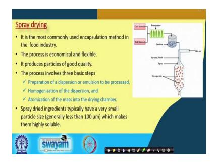
Spray drying: It is the most commonly used encapsulation method in food industry. The process is economical and flexible. It produces particles of good quality. The process involves three basic steps like, preparation of a dispersion or emulsion which is to be processed it is followed by homogenization of the dispersion and finally, atomization of the mass into the drying chamber.
