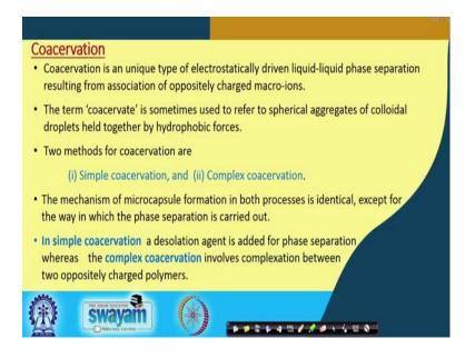
The other technology is the coacervation. Coacervation is a unique type of electrostatically driven liquid-liquid phase separation resulting from association of oppositely charged macro-ions. The term coacervate is sometimes used to refer to
