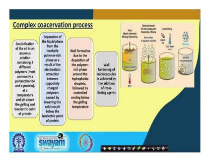
Complex coacervation process: In the first step, the emulsification of the oil in an aqueous solution containing two different polymers generally polysaccharides and a
