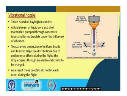
The vibrational nozzle technology is based upon the Rayleigh instability in this process. A fluid stream of liquid core and shell material is pumped through the concentric tubes and forms droplets under the influence of vibration.
