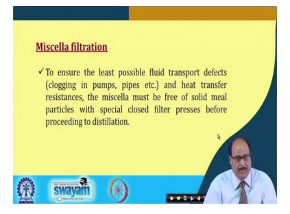
Apart from distillation, another important operation is the miscella filtration and it is done to ensure the last possible fluid transport defects, like clogging of the pumps, pipes etc. and heat transfer resistances. The miscella must be free of solid meal particles with special closed filter presses before proceeding to distillation.
