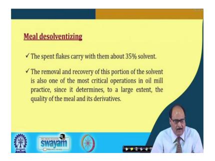
The spent flakes contain around 30 to 35 % solvent. So, it becomes very important operation that these solvents should be recovered from the meal which can be recycled and reused. The meal can be used for different food purposes. So, removal and recovery of the solvent is one of the most critical operation in oil mill.
