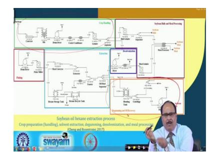
This figure commercial plant extraction facility is shown starting from the handling of the material (whole seed) until oil and meal are obtained. It is basically for soybean oil extraction and meal processing, but can be used for any other oilseeds or nuts.
