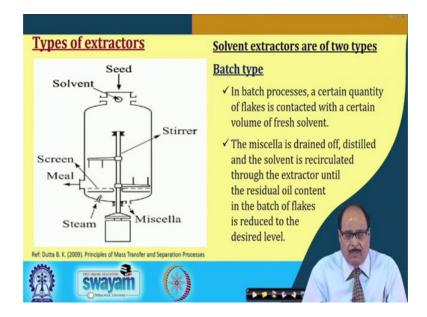
The porous mass is fed to the solvent extractor. The proper conditions of temperature, pressure etc. are maintained and there is an intimate contact of the prepared mass with the solvent. Solvent flows and penetrates into the mass; the oil dissolves into it and then it comes out along with the solvent.
