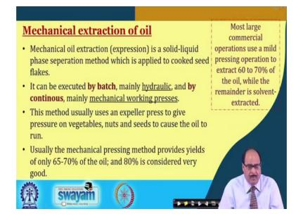
After these pretreatments, the prepared oilseeds are crushed, cooked and conditioned oilseeds are subjected to mechanical extraction process. So, the mechanical extraction process or expression is a solid-liquid phase separation method which is applied to cooked seed flakes. It may be executed in batch, mainly by hydraulic presses or in continuous operation by mechanical working presses.
