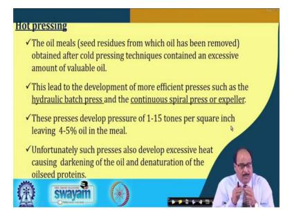
So, to overcome this or to get more oil yield, hot pressing methods are developed. The oilseed meals (seed residues from which oil has been removed) obtained after cold
