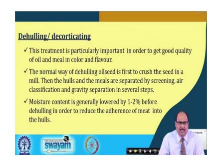
After the cleaning, the seeds are dehulled and decorticated i.e. outer husk or fibrous materials of the seed or seed coat is removed. And this treatment is particularly important in order to get good quality of oil and meal in terms of colour and flavour. The normal way of decorticating oilseed is first to crush the seed in a mill. Then the hulls and the meals are separated by screening, air classification and gravity separation in several steps as the case may be.
