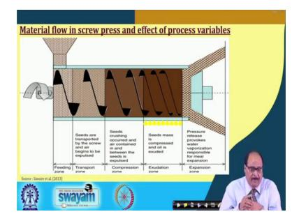
Material flow in screw press and effect of process variables:
