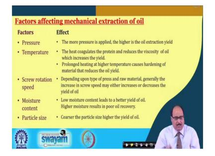
Factors affecting the mechanical extraction process of the oil and yield: Particularly if the more pressure is applied, the higher is the oil extraction yield. The heat coagulates the protein, reduces the viscosity of the oil, which increases the yield. Prolonged heating at higher temperature, however causes hardening of the material that reduces the yield. So, excessive heating should be avoided.
