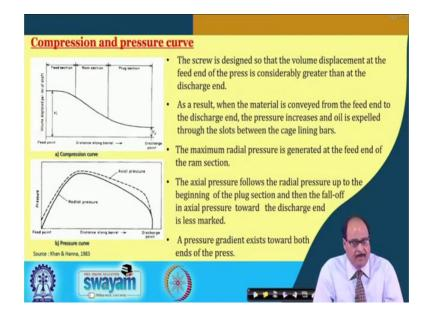
Compression and pressure curve: It was reported that the screw is designed (see Fig.), so that the volume displacement at the feed end is considerably greater than that at the discharge end. As a result, when the material is conveyed from the feed end to the discharge end, the pressure increases and oil is expelled through the slots between the cage lining bars. The maximum radial pressure is generated at the feed end of the ram section.
