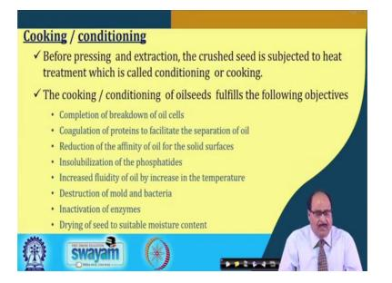
The next pretreatment is cooking or conditioning. So, before the extraction process, the crushed seed is subjected to heat treatment and this process is called conditioning or cooking. Cooking serves the following objectives:
