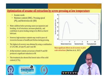
Optimization of sesame oil extraction by screw-pressing at low temperature:
