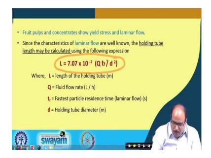
Fruit pulps and concentrates show yield stress and laminar flow. And, since the characteristics of laminar flow is well known, the holding tube length can be calculated using this formula:
