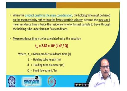
When the product quality is the main consideration, the holding time must be based on the mean velocity rather than the fastest particle velocity because the measured mean residence time is twice the residence time for fastest particle to travel through the holding tube under laminar flow conditions.
