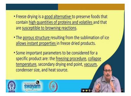
Freeze drying is a good alternative to preserve foods that contain high quantities of proteins and volatiles and that are susceptible to browning reactions. The porous structure resulting from the sublimation of ice allows instant properties in freeze dried products. Some important parameters to be considered for a specific product are: the freezing procedure, collapse temperature, secondary drying end point, vacuum, condenser size, and heat source.
