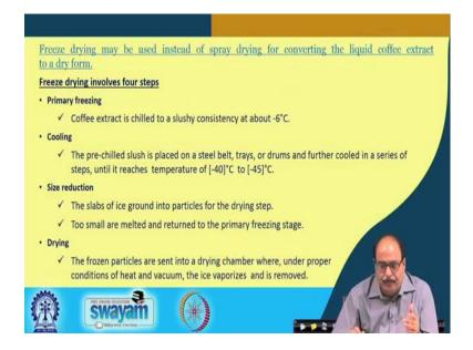
Freeze drying may be used instead of spray drying for converting the liquid coffee extract to a dry form.
