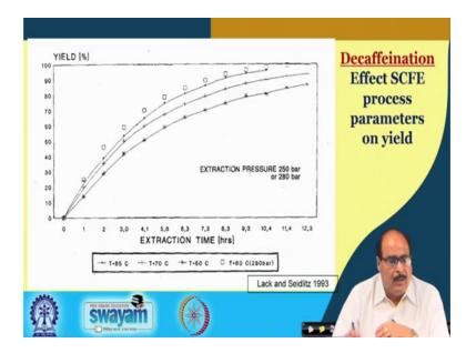
The extraction process variables i.e. extraction pressure, time, and temperature influence the yield of the caffeine. Y-axis (in graph) is the yield of the caffeine that increases with the increase in the time, temperature and pressure. For maximum yield or maximum recovery one should always standardize the process and optimize it.
