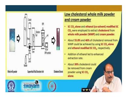
Low cholesterol whole milk powder and cream powder: SC CO<sub>2</sub> alone and ethanol modified CO<sub>2</sub> were employed to extract cholesterol from whole milk powder (WMP) and cream powder. About 55.8 % and 46 % of cholesterol removal from WMP could be achieved by using SC CO<sub>2</sub> alone and ethanol modified SC CO<sub>2</sub> respectively. Addition of ethanol led to enhanced extraction rate.
