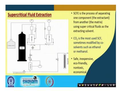
Supercritical fluid extraction (SCFE) is a process of separating one component from the other using supercritical fluid as the extracting solvent. The component which is separated is known as extractant and the material from which it is extracted is known as a matrix.
