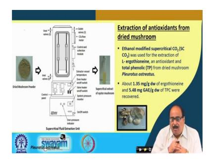
Extraction of antioxidants from dried mushroom: The mushroom is taken, dried and made into the powder. Then in the powder form, it is introduced into the extraction vessel and the rest thing follows as usual like in any other process. It is given the desired time to contact with super critical carbon dioxide at desired temperature and pressure. Finally, ergothioneine 1.35 mg/g dry weight and total phenols about 5.48 mg GAE/g dry weight have been obtained.
