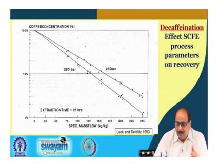
In the graph, it is shown that the concentration of the material which is extracted i.e. caffeine is initially taken as the 100 % concentration which was fed into the extractor and the extraction time maintained was 12 hours. The concentration of the material that is remaining increases with both increase in the mass flow rate (kg per kg solid) as well as the pressure.
