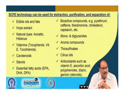
SCFE is applied for extraction, purification and separation of edible oils and fats, hops extracts used in the beer making industry. Hops is a flowering part from which the flavouring component is extracted that gives the characteristic flavour to the beer.
