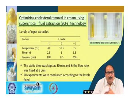
For optimization, the input variables were temperature (40-75 °C), time (2.5-3.5 h) and pressure (100-250 bar). About 20 experiments having combinations of these variables were conducted as per the experimental design; the static time was kept 30 min and the flow rate was fixed at 6 l/min.
