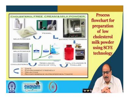
Process flow chart for the preparation of low cholesterol milk powder using SCFE technology: In the pictorial flow diagram, the milk powder is introduced into the extraction vessel and this vessel is fitted in to the SCFE equipment. The characteristics of low cholesterol dairy cream and milk powder obtained were also analyzed and found that
