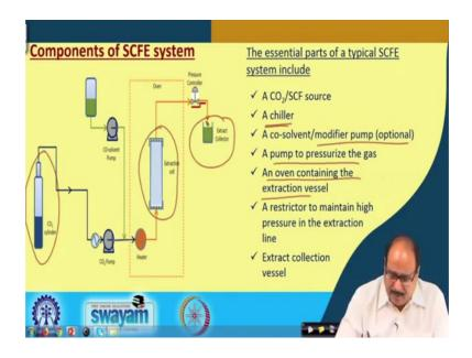
Components of Supercritical Fluid Extraction system:
