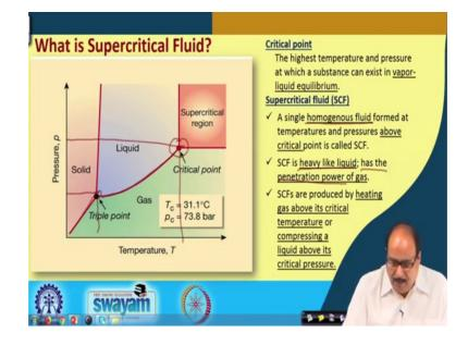
Supercritical fluid: In graph (pressure vs temperature) shown, a critical point can be observed which is the highest temperature and pressure above which a material can exist
