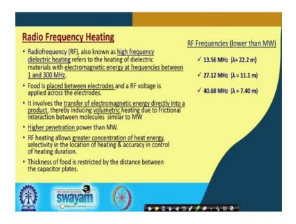
RF heating is also known as high frequency dielectric heating. It refers to the heating of dielectric materials with electromagnetic energy at frequencies between 1 and 300 MHz.
