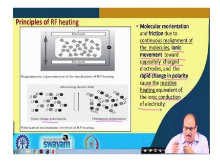
The principle of radio frequency heating is almost similar to that of the microwave heating. Here, space charge polarization or orientation polarization are the phenomena. The molecular re-orientation and friction due to continuous realignment of the molecules or ionic movement towards the oppositely charged electrodes, and rapid change in polarity cause the resistive heating equivalent of the ionic conduction of the electricity.
