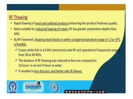
Radiofrequency assisted thawing becomes a rapid means of thawing of meat and sea foods. It enhances the product freshness and quality; it is more suitable for industrial heating of meats. Radio frequency has greater penetration depth than the microwave. By suitable RF treatment, thawing of meat block to within a target temperature range of -1 to +5 °C is feasible i.e. without much increase in the temperature of the muscle, thawing is possible.
