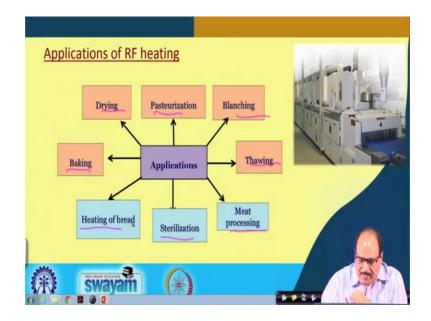
It can be applied extensively in various food process operations for preservation purposes, for preparation of products, and for improvement in the quality and process efficiency. It has common applications like in any other heat process, it can also be used for drying purposes, pasteurization, blanching, thawing, meat processing, sterilization, baking or even toasting of the bread, etc.
