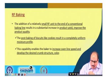
Radio frequency heating has a good application in baking industry. The addition of a small RF unit to the end of conventional baking line results in substantial increase in the product yield and improves the product quality. The post baking of biscuits like cookies etc. results in uniform moisture profile in the product. This capability enables the baker to increase the oven line speed and develop the desired crumb structure and even desired color, texture in the products.
