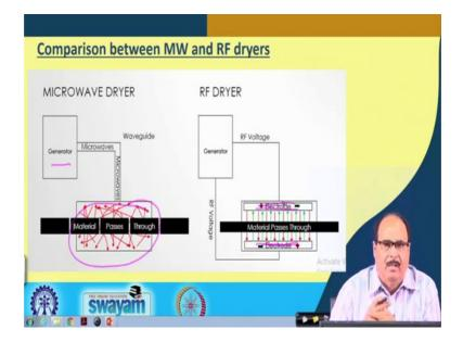
It is a pictorial comparison between the microwave and radio frequency dryers. MW dryer has a generator and through this, microwaves are generated with the help of
