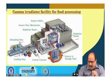
The figure shows a gamma irradiation facility for the food irradiation. Gamma irradiation source cobalt 60 is kept in storage in the deep pool of the water. The food material depending upon its type in the packaged or unpackaged form is exposed to the irradiation.
