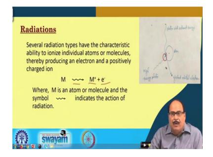
There are several radiation types which have the characteristic ability to ionize individual atoms or molecules, there by producing an electron and a positively charged ion. In this figure, high energy photon bombards the atom and excites the electron by absorption of energy. This electron gets ejected from the orbital resulting in a positively charged atom. Compton effect shows that when atom is bombarded by irradiation, positively and negatively charged ions are produced.
