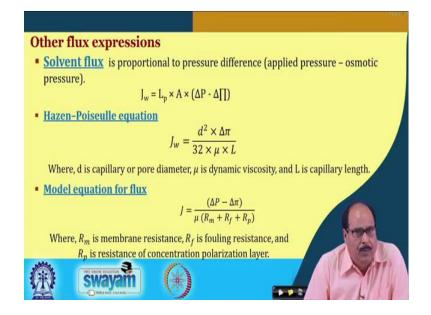
There are few other calculations which need to be taken into consideration for better process efficiency. Solvent flux is proportional to the pressure difference i.e. applied pressure minus osmotic pressure.
