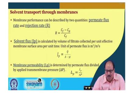
In solvent transport phenomena through membranes, two important properties should be considered. One is permeate flux and another is the rejection rate i.e. what is the amount of the permeate that is allowed to pass through the membrane and what are the components that are rejected by the membrane.
