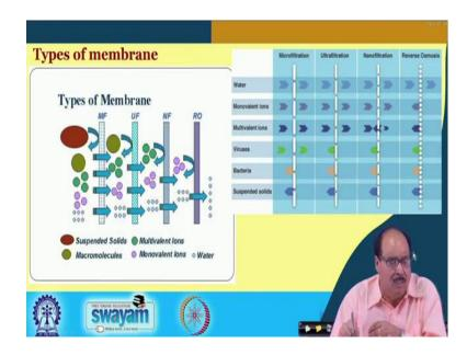
Depending upon the nature of the molecules or atoms which are to be separated by these processes there are different types of membranes:
