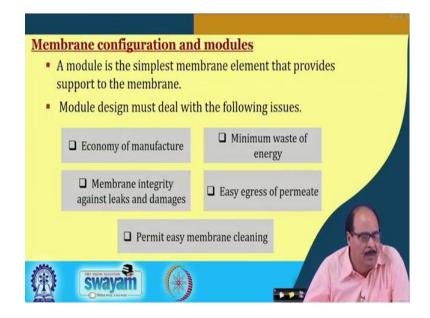
A module is the simplest membrane element that provides the necessary support for keeping the membrane in normal place. Of course module design must deal with the aspects like economy of the manufacture. There should be minimum waste of energy, membrane integrity against leaks and damages, easy egress of the permeate and it should permit easy membrane cleaning. So, the membrane module should have these characteristics.
