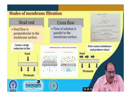
There are basically two types of flow: one is the dead end flow; another is the cross flow. In the dead end flow, the feed flows perpendicular to the membrane surface. This type of flow normally is used in batch processes and it has some problems particularly regarding fouling and concentration polarization as the solute particles tend to get deposited on the surface of the membrane, causing a large reduction in flux.
