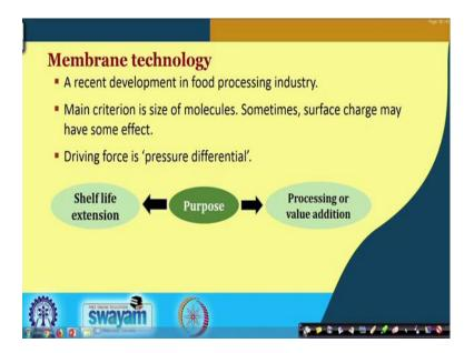
Membrane technology is a comparatively recent development in food processing industry. Major criterion of this technology is separation on the basis of size of the molecules. Sometimes even surface charge may also have some effect. The driving force is generally the pressure differential. There are two main purposes of this technology; processing or value addition and shelf life extension.
