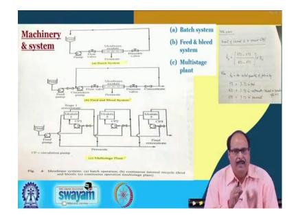
It was the invent of the cross flow system which facilitated the application of membrane technology in the industrial or commercial processes.
