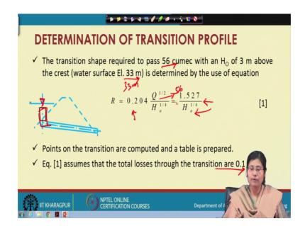
So, once we obtain the crest profile and now we determine the transition profile. So, this is a transition profile. So, crest profile was this, the top point panel. So, this design was completed. Now the second part the transition profile, the transition shape required to pass the 56 cumec that was the design discharge with an H 0 of 3 meter above the crest.
