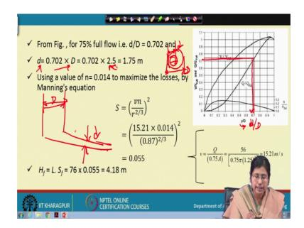
Now, since the pipe is 75 percent full. So from this graph, so, this is the ratio between v by v full and for different depth. So, 75 percent full. So, you can take the point here and here. So, this is 75 percent full.
