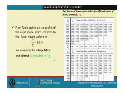
So, the value of Hs by Rs is 1.41 now. So, for different value of Hs by Rs, so this table that is given, so between 1 and 2.
