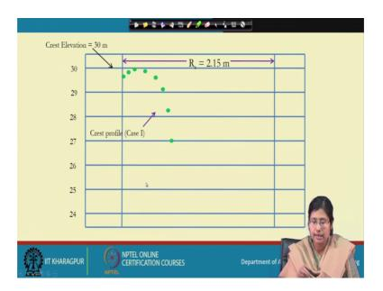
So, at a crest elevation of 30 meter and at a different value of X and Y and Rs, the radius at the inlet is 2.15 meter was kept and we can get the crest profile like this after interpolating this table values.
