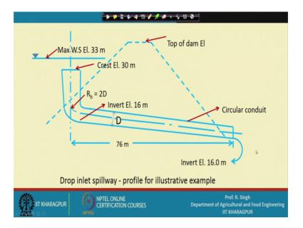
So, now this is the basic diagram. So, here the maximum elevation since, H 0 is assumed as 3 meter, sorry. So, here it says the H 0, the surcharge head is 3 meterand the 30 meter.
