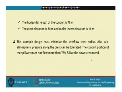
So, what are these conditions? So, the horizontal length of the conduit is assumed that 76 meter and a crest elevation is given 30 meter and outlet invert elevation is 16 meter.
