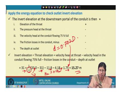
Now, we apply the conservation of energy equation to check the outlet invert elevation. So, here the in elevation at a throat is positive and the pressure head at the throat. So, this has to be negative. So, we are deducting this velocity head at the conduit assuming the pipe is 75 percent full. So, you will have to deduct it, because this is a head loss, the frictional losses at the conduit.
