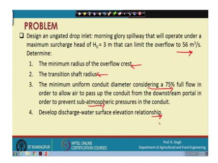
So, this is the problem statement. So, design an ungated drop inlet and here we are going to take morning glory spillway kind, that will operate under a maximum surcharge head H 0 as 3 meter, that can limit a overflow of 56 cumec.
