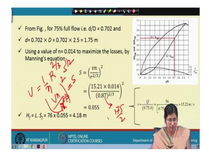
Now, this is this universal equation, the velocity of flow through open channel. So using that so, you can get the value of S; so, V n square.
