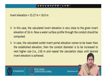
Now, the invert elevation was given in the design problem is 16 meter, which is very close to 15.27 meter.
