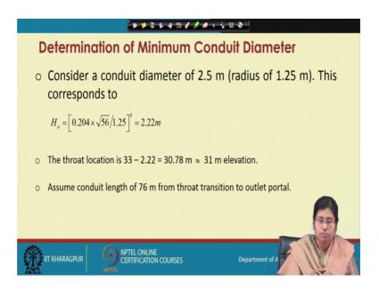
Now, the next part is the determination of the minimum conduit diameter. So, first we assume a known conduit diameter, say 2.5 meter, which is standard since the diameter is 2.5 meter, the radius is half of that. So, this is the 1.25 meter is obtained like this and this corresponds to. So, we again plug into the basic equation.
