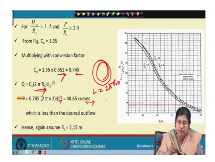
So, for this ratio of 1.5 meter and assuming the ratio P by Rs as greater than 2, so, if it is 1.5 meter, sorry;so what is the corresponding value of this coordinate here? So, is to determine the coefficient of discharge here, so, the C 0 value is 1.35 meter. Since this graph is prepared in MK's unit. So, we multiply using a correction factor to convert it into SI unit. So, the conversion factor is nothing but 0.552 here.
