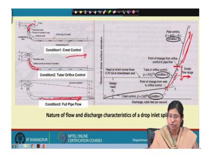
And now this particular figure shows the nature of flow and discharge characteristics of drop inlet spillway. So, here in the flow of drop inlet spillway; so, three condition prevail. So, first is condition 1 that is a crest control, when the water enters through the crest and the second is when it flows through the tube or the transition phase when tube or orifice control takes place and the third is the full pipe flow conditions, so, which is the last part.
