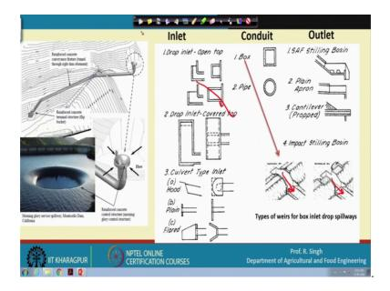
So, this is a drop inlet spillway. So, here you can in the left side you can see a morning glory service spillway. So, this is in one of the structure located in Monticello dam in California and here you can see the reinforced concrete conveyance feature or the tunnel through the right abutment of the dam. So, from here the morning glory spillway takes the water here and then it goes here. So, here the flow of water takes place and these are
