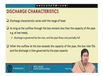
Now, coming to discharge characteristics, discharge characteristics varies with the range of head, second as long as the outflow through the box remains less than the capacity of the pipe example, at low heads. So, discharge is governed by the riser and the pipe flows only partially full. Third when the outflow at the box exceeds the capacity of the pipe the box inlet fills and discharge is then governed by the pipe capacity. So, these are some the special some of the discharge characteristics.
