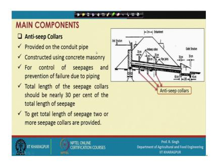
Now coming to the main component; so, here we are going to cover some of the main component of this drop inlet spillway. So, first one is anti seep collars. So, you can see, so here is the inlet structure here is the complete the conduit part and this is a outlet. So, in the conduit structure or the conduit pipe structure is a anti seep collars are provided. So, you can see the small collars are provided here.
