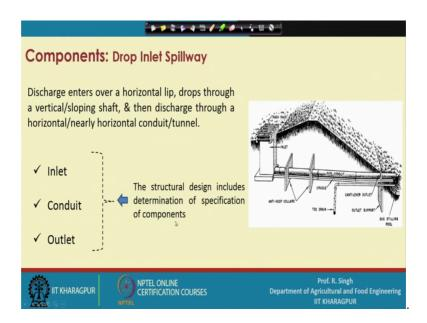
Now coming to the design, the structural design include that is determination of the specific components as I described earlier.
