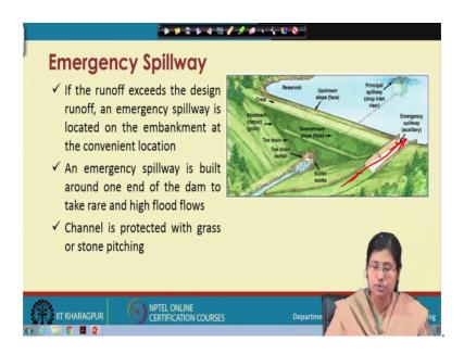
Now, it also consists of an emergency spillway. So, if the runoff exceeds the design runoff, so, as here in this case an emergency spillway is kept, which is located at a embankment at a convenient location.
