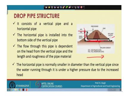
Now coming to the drop pipe structure; so, here at the right side you can see the drop pipe structure. So, this is one of the drop pipe structure. So, here is a free board is
