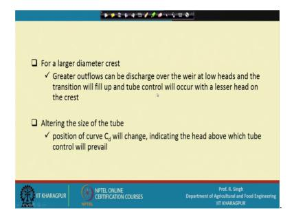
Now, for a large diameter crest greater outflows can be discharge over the weir at low heads and the transition will fill up and tube control will occur with a lesser head on the crest. Now, altering the size of the tube the position of curve C d will change, where c d is the coefficient of discharge indicating the head above which tube control will prevail.
