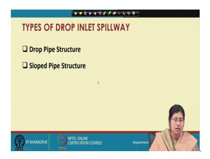
Now, what are the type of drop inlet spillway? So, there are basically two types. So, first is drop pipe structure and the second one is slopped pipe structure.
