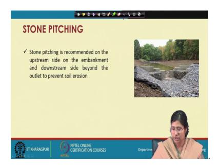
Now, as you can see this is a emergency spillway structure here and there is a stone pitching is provided to reduce the flow of water or the velocity of flow. So, stone pitching is recommended on the upstream side of the embankment and the downstream side beyond the outlet to prevent soil erosion because of the high flow of the water. So, the stone pitching is provided.
