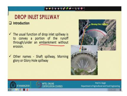
So, what is drop inlet spillway? So, drop inlet spillway is a kind of spillway where the function is to convey the portion of runoff through or under the embankment without any erosion.
