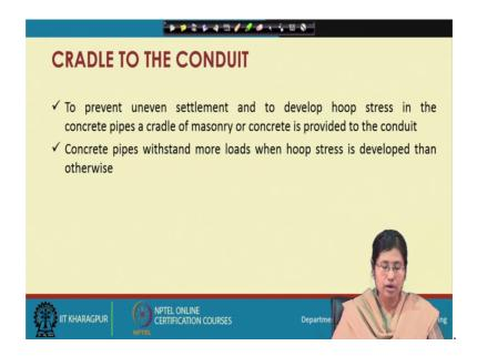
Now, cradle to the conduit to prevent uneven settlement and to develop hoop stress in the concrete pipe a cradle of masonry or concrete is provided to the conduit. So, concrete pipes withstand more loads when hoop stress is developed then otherwise. So, when the concrete pipes are provided when the hoop stresses developed in the system.
