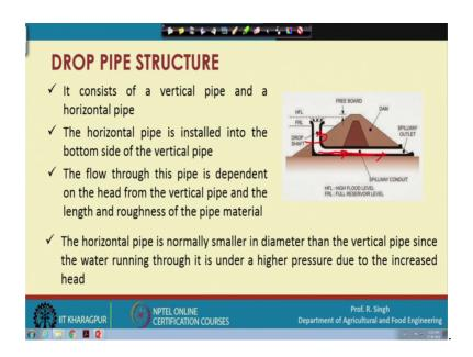
That you can say the diameter of this horizontal pipe is much lesser in diameter than the vertical pipe, why? Since the water running through it is under at high pressure and due to high since the water is flowing through it at a high pressure. So, increased head prevails so, the diameter of this is kept smaller than the vertical pipe.
