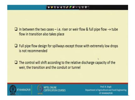
Now, in between the two cases that is riser or weir flow and the pipe flow tube in that case the tube flow in transition also takes place. And Secondly, full pipe flow design for spillways except those with extremely low drops is not recommended and third the control will shift according to the relative discharge capacity of the weir, the transition and the conduit or tunnel.
