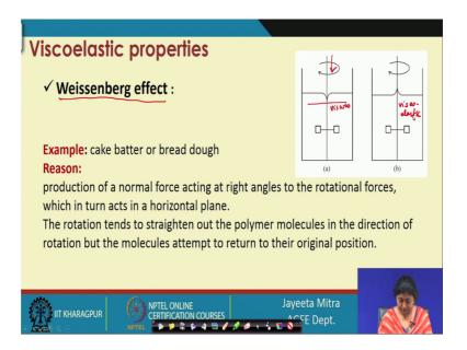
So, we will see an interesting phenomena here, viscoelastic material which is having some special property, which is visible compared to the viscous material. So, if we take a rod, if we dip one rod into a viscous material and give a rotational movement to it then we will observe a vertex in the liquid ok. So, it is clearly visible.
