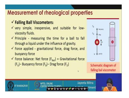
So, next is the falling ball viscometer, falling ball viscometer also very common and we can we can see the diagram, how we measure it; we take a cylinder and fill it with the fluid for which we want to measure the viscosity and here the criteria is that, we should take at least the particle ten times smaller than the diameter of the this tube to get the wall effect neglected.
