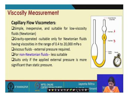
So, let us first take the case of capillary flow viscometer. This is the pictorial representation of a capillary flow viscometer; however, we may find that different kind of you know pictures, different kind of representation keeping the basic principle intact. So, it is very simple, inexpensive and it is suitable for the low viscosity material. It is not that much suitable for the high viscosity. What happened that in case of capillary viscometer?
