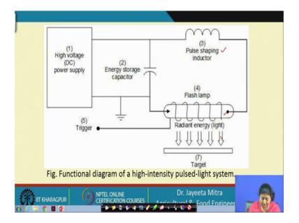
So, this is the system here we have the high voltage DC power supply; we have a capacitor energy storage capacitor that stores the in energy and when we apply the switch? So, the flash lamp here it starts generating the intense intensity of the light from the low to high and a flash will be generated.
