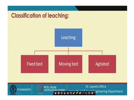
Now, coming to the classification of leaching so, leaching can be broadly categorized as either fixed bed leaching, moving bed leaching or agitated. So, fixed bed leaching; that means, the bed of the particle is fixed through which the solvent is passing, and within this pass 1 pass or 2 pass like that the material the solute will be extracted.
