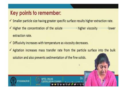
So this we have already discussed that the smaller particle having higher greater affinity greater extraction, concentration higher the concentration of the solute higher the viscosity lower will be the extraction rate that is very important. And diffusivity increases with temperature as viscosity decreases and agitation increases so, mass transfer will increase.
