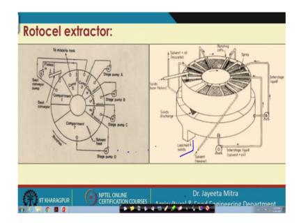
So, this is again the schematic view of Rotocel extractor we can see there is component 1, 2, 3, 4, 5, 6 and 7, I am solving feed at every from the top section everywhere the solvent feed is entering into and there are pumped to flow the material from one stage to the other. After one stage of extraction it is being thrown to the next one. So, like that an at the end of the process from the bottom the leach solid is being collected, ok.
