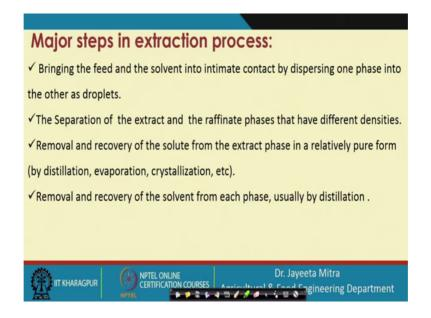
So if you look into the major steps in extraction process, you can categorize them into many segments. So, first is bringing the feed and the solvent into intimate contact by dispersing one phase into the other ok. So, the feet and the solvent you have to bring into intimate contact by dispersing one phase into the other as the droplets. So, the separation of the extract and the raffinate phase that how different density.
