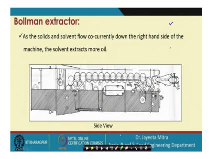
So, there are different geometry this is the side view of Bollman extractor. The mechanism is same as we have explained.
