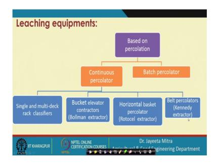
Now, based on the percolation again we can divide them into continuous percolator batch percolator, and continuous can be also divided into single and multi-deck rack classifiers. Bucket elevator contractor that is called the Bollman extractor, horizontal basket percolator that is called Rotocel extractor, and belt peculator that is called the Kennedy extractor.
