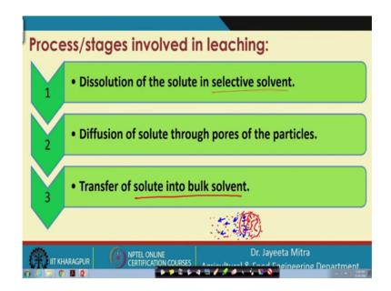
So, if we specifically see leaching methods so, in that these are the steps that we normally observe, once we make the once we bring the product bring the solid material, from which we want to extract the particular compound or particular solute. So, when that comes into contact with the solvent, solvent has to mix with that material very well and has to penetrate or percolate through it properly through the solid material solid phase properly.
