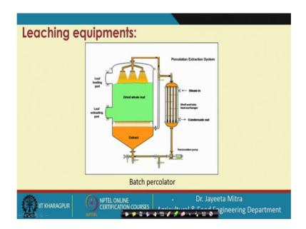
So, the batch percolator if you see this is a batch percolator. So, here there is loading section there is a loading port, and there is an unloading port ok. So, material is loaded from here and unloaded from here. We have a percolation extraction system where the spray of the solvent is from the top, and while passing through while percolating through the bed of the particle, the extraction is being done and then it is extracted at the bottom.
