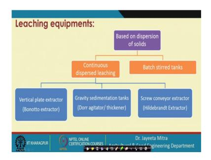
Now, another classification we can develop based on the dispersion of solid that is continuous disperse leaching and batched stirred tanks continuous disperse leaching again can be classified as vertical plate extractor that is called Bonotto extractor. Gravity sedimentation tank that is called Dorr thickener or agitator and the last one is the screw conveyor extractor that is called Hildebrandt extractor.
