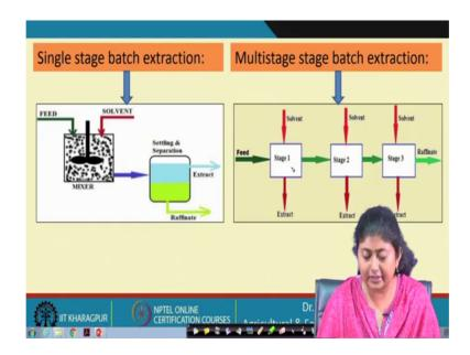
So, in the single stage batch as we have in the very beginning of this class this, this chapter we mentioned that in the feed and solvent comes into chamber comes into at the mixture chamber. There is proper mixing by paddles or agitators. And then settling and
