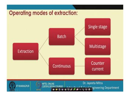
Another operating mode we can think of out that is the extraction of other batch or in continuous mode, in batch that is single stage multi stage and counter current stage.
