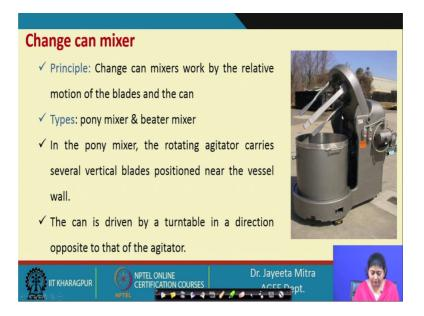
So, first you see the change can mixer. The principal is change can mixer work by the relative motion of the blades and the can. So, the type is pony mixer and beater mixer, in the pony mixer the rotating agitator carries several vertical blades positioned near the vessel wall. The can is driven by a turntable in a direction opposite to that of the agitator.
