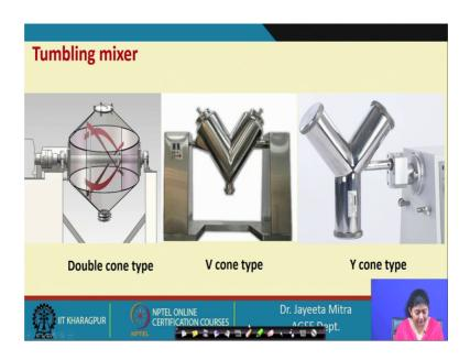
Double cone type is this one and there is a spiral blades are also there, which will help you to initiate proper mixing and there is V-cone type. So, V-cone type is this one and these are also can be revolved freely. There is a Y-cone type mixer, this there is a 3 1 extra cylinder added to V-cone and this will also have give some extra volume and a better mixing.
