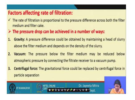
Now, coming to the factors affecting the rate of filtration. So, the rate of filtration is proportional to the pressure difference across both the filter medium and the filter cake. So, the pressure drop can be achieved in a number of ways first one is gravity, where a pressure difference could be obtained by maintaining a head of slurry above the filter medium and depend on the density of the slurry.
