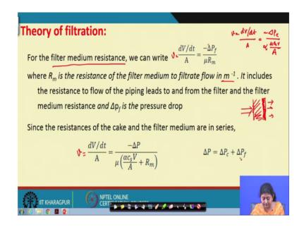
Now, for the filter medium resistance what we can write? We have seen now then how filter cake resistance can be formed, but definitely some resistance will be provided by the filter medium as well. So, for that what we will do is we use a factor R m. So, similar manner that way we did we calculated for the filter cake that is v is equal to dV by dt divided by A that is equal to minus delta P c by alpha into mu c s v by A.
