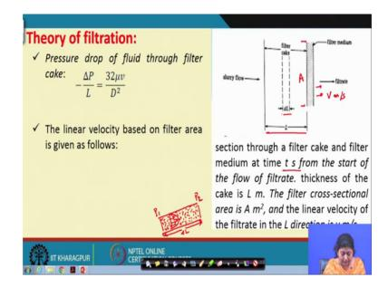
Now, coming to the theory of filtration, that is what is the mechanism behind filtration. So, here we will assume that with start of the filtration if we continue it for a time, let us say t second then the deposition of cake will occur and the length of that deposition let us say L meter.
