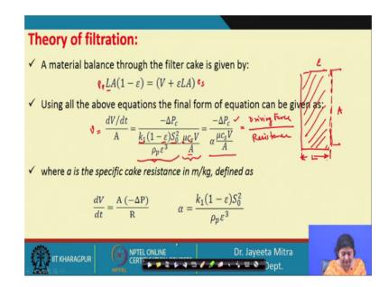
So, how we can develop that first we have seen that what will be the flow of fluid through that; that means, about the filtrate that has been passed through. Now, we try to establish a material balance to get some idea then how the deposition of cake has occurred.
