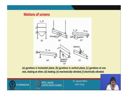
Now, motion of screen can be of many types; are the first one is the gyration in horizontal plane figure a, b is the gyration in particle plane, c the eccentric gyration. So, gyration at one end shaking at the other end; gyration at one end and shaking at the other end, d is shaking only and e is the mechanically vibrated screen and f is the electrically
