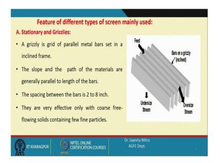
Now, feature of different types of screens mainly used that is first one stationery and grizzlies. A grizzly is grid of parallel metal bar set in a in client frame. As we can see here the parallel metal bars are there those are set on an inclined frame from one side series entering and the undersized which is passing through the screen that is come from the down section and the over size is moving with the stream.
