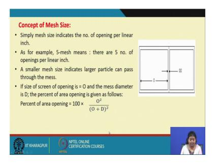
Now what is mesh size? We are since the last class we are we are talking about 400 mesh 20 mesh or 200 mesh like that. So, these are specification that we generally used for describing a particular kind of mesh. Simply mesh size indicate the number of opening per linear inch; as per example 5 mesh means there are 5 number of openings for linear inch.
