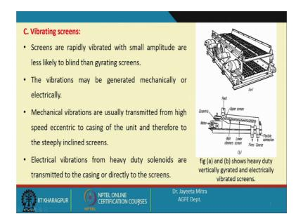
Now, vibrating screen; so, this is another screen layer which can be vibrated horizontally or vertically. So, this screens are rapidly vibrated with small amplitude and are less likely to blind the blind that gyrating screens. So, because of this vibration, small amplitude vibration that we are providing the screens are less likely to blind than the gyrating screen.
