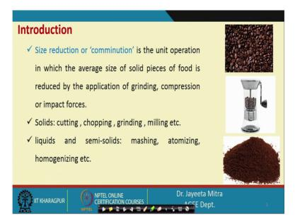
Size reduction or comminution is the unit operation in which; the average size of the solid pieces of the food is reduced by the application of grinding, compression or impact forces.
