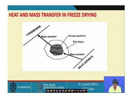
So, in case of freeze drying, let us say first we have a food sample and we first freeze it by lowering the temperature. So, all the moisture in the food become frozen, converted to ice and after that we will apply heat source we will apply heat to the material, so that as the heat will be transferred to the frozen layer, it will directly sublime under that reduce vacuum condition and that will be taken out by a vacuum pump.
