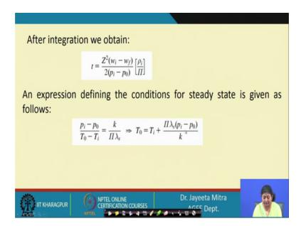
So, here also after integrating we are getting this that t will be equal to Z square w i minus w f by 2 into p i minus p 0. Here also we are integrating with in z equal to 0 at t equal to 0 to z equal to Z at t equal to time t. So, here we are getting this factor multiplied with rho i by capital pi. So, an expression defining the condition for steady state is given as follows where p i minus p 0 by T 0 minus T i that will be equal to k by pi into lambda s.
