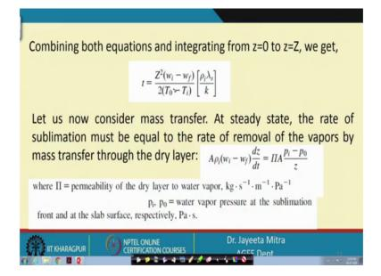
So, for this equation, if we integrate from z equal to 0 at time t 0 to z equal to Z at time t, we can get t equal to Z square w I minus w f divided by 2 into T 0 minus T i into rho i lambda s by k ok. So, now, if we consider the mass transfer at steady state, the rate of sublimation must be equal to the rate of removal of the vapors by mass transfer through the dry layer.
