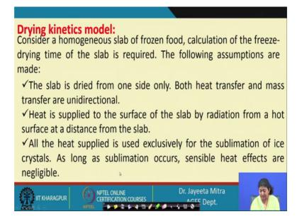
So, drying kinetics model; now, what we can do as most of the cases for this time for this kinetics development, we will consider we will try to consider a steady state case that means whatever heat we are providing to the frozen layer that will be utilized for sublimation of the ice front and we consider of course, no heat loss. And a homogeneous slab we have taken here of frozen food and we will calculate the freeze drying time of the slab.
