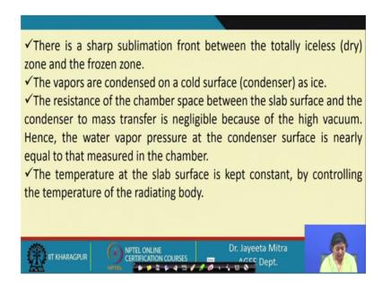
The temperature at the slab surface is kept constant by controlling the temperature of the radiating body.
