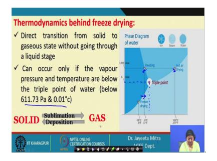
So, now we will see that how or what is the principle of this freeze drying. Here we can see the phase diagram of water. So, there we can see the all three phases solid liquid and gas solid liquid and gas this three phases are there and triple point which is the point where all three phases coexist right. So, we need to perform the operation somewhere below this point so, that we can directly convert ice to vapor.
