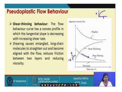
So, as I mentioned that shear thinning behaviour, where we can we can observe that the apparent viscosity is decreasing with increasing shear rate. So, this is shown by this strain; so apparent viscosity here we are plotting eta that is equal to K into gamma dot to the power n minus 1.
