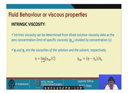
So, intrinsic viscosity; what is it intrinsic viscosity can be determined from dilute solution viscosity data as the 0 concentration limit of specific viscosity eta sp divided by the concentration C. So, eta and eta s are viscosity of the solution and the solvent respectively. So, eta is limit concentration tends to 0 eta sp by C and eta sp equal to eta that is the viscosity of the solution minus eta s that is viscosity of the solvent divided by eta s.
