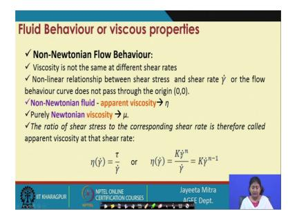
So, non-Newtonian flow behaviour that is viscosity is not the same at different shear rate non-linear relationship between shear stress and shear rate gamma or the flow behaviour curve does not pass through the origin. That is another case happen in case of bingham plastic fluid ok.
