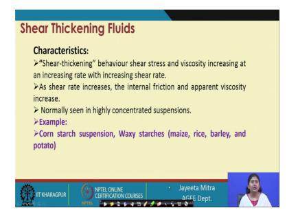
The reverse strain that is shear thickening which is the behaviour where shear stress and viscosity increasing at an increasing rate with increasing shear rate. So, normally this is seen in high concentrated suspension; for example, corn starch suspension waxy starch that is maize, rice, barley and potato.
