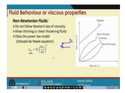
So,; so they do not follow the Newton's law of viscosity shear thinning and shear thickening fluid and they obey the power law model this is also called the Ostwald-de Waele equation; that is tau yx is equal to K into dvx by dy to the power n.
