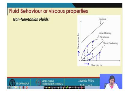
So now non-Newtonian fluid; so, here is the plot that shear rate and shear stress we have plotted in x and y direction respectively. So, the straight line the straight line where the slope constant that comes under Newtonian you know that already. Now these 2 plot where we are getting one curve that is changing its slope at every instant of changing in the shear rate and as shear rate increases ok.
