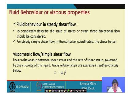
So, now fluid behaviour in steady shear flow; so, to completely describe the state of stress or strain three directional flow should be considered for steady simple shear flow. In the Cartesian coordinates, the stress tensor is used to express the flow as I have mentioned already in the last class.
