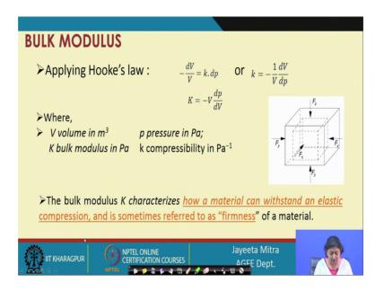
So, the bulk modulus k characterizes how a material k can withstand and elastic compression and is sometime referred to as firmness ok. So, first one that is Young's modulus that is the concept of stiffness we are getting there. Here what we are getting that is concept of firmness, which is how a material can withstand and elastic compression elastic compression.
