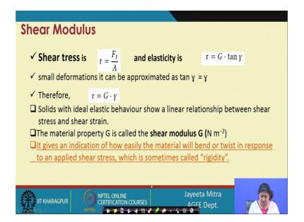
So, shear stress is expressed as tau equal to Ft by A ok. So, this is a you know tangential force is Ft by area. So, this force is acting parallel to the surface where as the normal forces that x on the perpendicular to the surface and the elasticity is tau equal to g into tan gamma. For the small deformation we can approximated tan gamma as equal to gamma therefore, we can write tau is equal to g into gamma ok.
