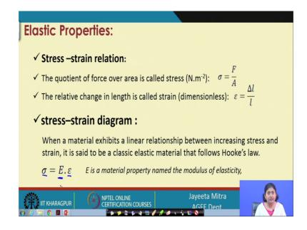
So, the elastic property of a material can be best understood by the relation between the stress and strain, and the coefficient of the force over area is call the stress expressed in Newton per meter square. So, sigma that is equal to F by A whereas, the relative change in length is called the strain, which is the dimensionless parameters of epsilon that is equal to delta l by l; so relative change of the length.
