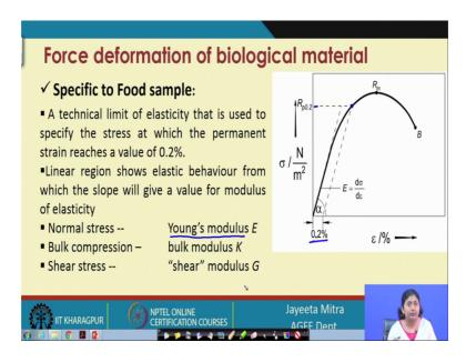
What happened in that case? For example, any food material the sharp change from the you know elastic to plastic state is not visible in case of the biological material. So, for that what we do is that if we see that how the plot is look like here the strain in percent we have plotted and stress is there. So, we can see that a gradual dome has been generated there is no transition point, there is no fixed yield point ok.
