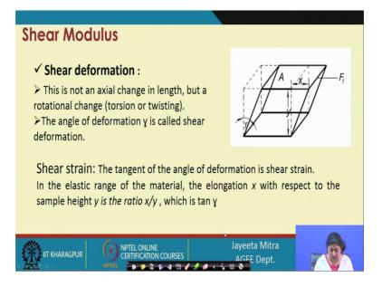
And another thing which is the shear modulus; so, what happened that as we have mentioned that if a dotted line dotted block is a stationary block kept on a surface and then we start pulling the upper plate with a with a force F t, then what will happen its try to bend towards the you know horizontal side it will it will be pulled down and an angle will be made from the equilibrium position. So, that is gamma.
