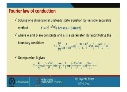
So, solving that one dimensional case; that is this equation delta T by delta small t that is equal to alpha d square t by d x square with these boundary condition and taking Y equal to T minus T 1 by T 0 minus T 1 we are getting.
