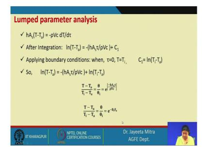
So, finally, we are getting this h into A s into T minus T a; that is equal to rho V volume of the body c, that is specific heat of the body into temperature, change of temperature with respect to time and we can integrate this equation. So, that we can get this term 1 n T minus T a; that is equal to minus h into A s into tau; that is time by rho into V c plus C 1
