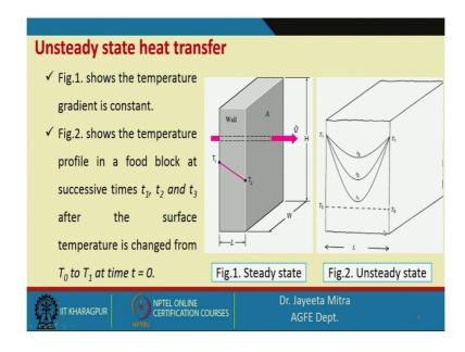
When we have reached the steady state ok, then we can see in this, in this picture where ok. So, in this picture we can see that its a slab of thickness L and width W height H through this Q dot amount of heat is flowing from the side where the temperature is T 1 to the other side where the temperature is T 2, because the gradient is from T 1 to T 2 as T 1 is higher temperature than T 2 a is the heat transfer area across which the heat flows.
