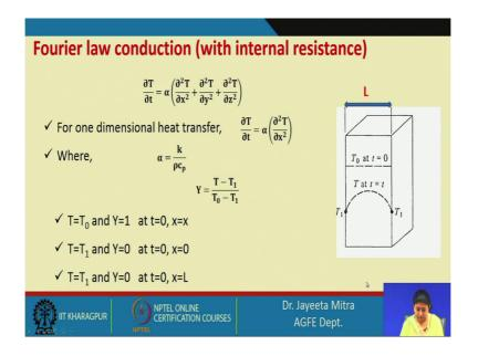
Now, next we will consider the Fourier's law of heat conduction for those material where the internal resistance exist, because the first case we have considered where the internal conductive resistance is negligible; that means, the thermal conductivity is very high. Now we will see the case with internal resistance. First we are taking the Fourier's law of heat conduction.
