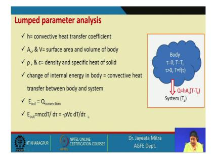
So, in case of lumped parameter analysis, as I said that initially when body was a fix temperature, where T equal to T i when time t equal to 0 and when time t greater than 0, Ts will be function of time. So, when this body is plunged into a sink having a temperature T a ok. So, heat will come out of the system. If this T a is lower than the body temperature or else
