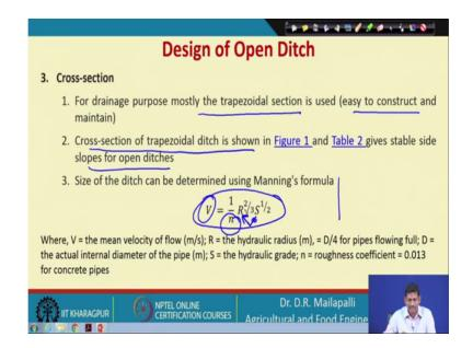
And the next is a; so, step number 3 so finding out the cross section area. So, for drainage purpose mostly the trapezoidal section is used because it is easy to construct and it can be maintained easily. And the cross section of trapezoidal ditch which is shown in figure 1 and figure 2, we are going to use in the next slide. Use the stable side slopes for open ditches ok.
