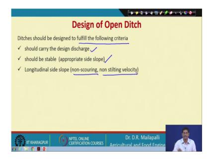
So the open ditch should designed to full fulfil the following criteria. The first one is should carry the design discharge so that is the I mean important parameter that is bare minimum. So, then should have stable side slopes and also longitudinal side slope for non-scouring the non-stilting velocity.
