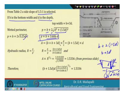
The remaining you know calculations from table 2 now, side slopes for I mean for these kind of salts alluvial soils is 1.5 is to 1. If b is the bottom width and d is the depth. So now, top width is equal to b plus 3 d because this is W1.5.
