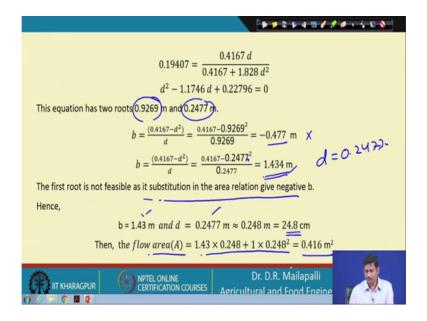
So, after simplification so you get the quadratic equation in d d square minus 1.1746 d plus 0.22796 is equal to 0. So, it has 2 roots so 1 is a minus 4 minus 0.477 and 1.434 this positive and negative. So, so since it has 2 roots, so sorry it has 2 roots there is a 0.9269 and 0.2477. So, substituting the one root into this.
