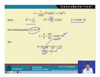
So, that will be so, this is the V and now R power 2 by 3 will be V by 1.79 substituting V value you get R is equal to 0.19407 these in meters from continuity equation Q equal to A into V.
