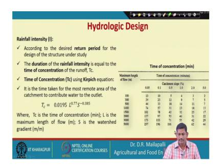
So, and the next is rainfall intensity. So, the third parameter rainfall intensity: so according to the desired return period for the design of the structure under this study. So, generally we are talking about the structure I mean we adopt the return period or the design procedure for designing a structure to soil conservation structures and similarly we use the rainfall intensity.
