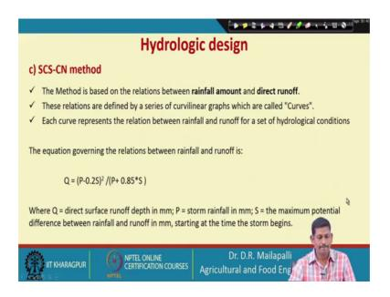
So, the next is SCS-CN method. So, that is a Soil Conservation Service Curve Number Method. So, the method is based on the relationship between rainfall amount and direct runoff.
