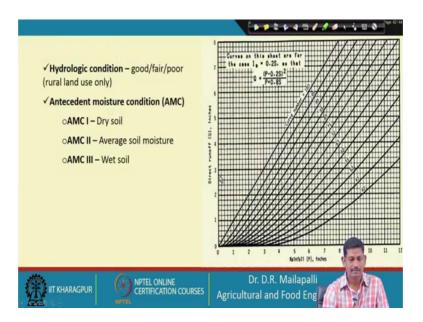
So, there is also table from where you can get the direct runoff. So, on x axis there is a rainfall knowing the rainfall and these lines are the curve numbers ok. So, curve number 100 and curve number 40 and y axis is a direct runoff. So, knowing the rainfall for example, 8 is the rainfall write on let us say on 65 curve number and then the corresponding runoff will be 4 inches here runoff will be 4 inches and here this is 8 inches.
