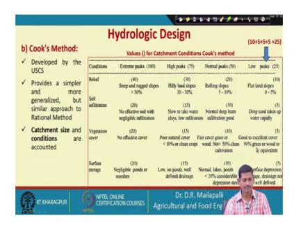
And Cook's Method: so the Cook's Method which is developed by USCS. So, this is United States Soil Conservation Service, USC SCS and it provides a simpler. So, this is a simpler than the Rational Method or you can also Cook's Method is a generalized Rational Method.
