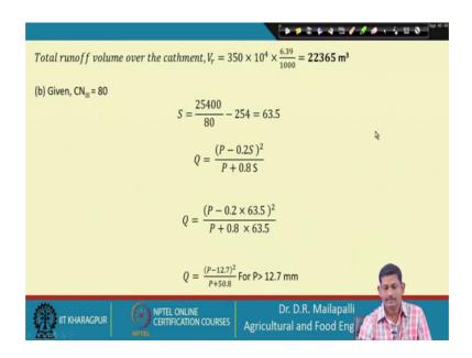
So, similarly for 80 right: so given curve number so find out S. So, that is 63.5, now substitute this 63.5 in this equation. So, now this is the equation. So, now, the Q value I mean P value should be at least 12.7. So now, from the table again we now bring the table and see and find out the.
