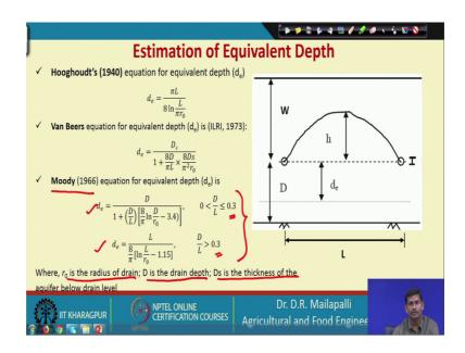
So, then Moody also has given an equation for equivalent depth. So, which is D by 1 plus D by L 8 by pi ln of D by r naught minus 3.4 and he have 2 conditions; so, 0 D by L less than equal to 0.3 and the D by L greater than 0.3. So, based on these 2 conditions so, d e will be estimated with different formulas. So, r naught is the radius of the drain and D is the drain depth ok; so, then D s is the thickness of the aquifer below drain level.
