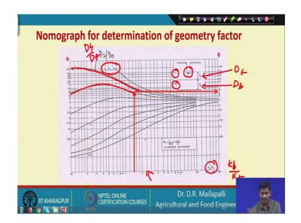
And then there is a Nomograph also available. So, here for example, this is the I mean the drain installation. So, the drain is at the top layer drain is at the top layer and K 1 top layer hydraulic conductivity, K 2 bottom layer hydraulic conductivity and D naught this is. So, the this D 2 is D b right, D 2 is D b and D naught is D t ok. So, this is D t and this is D b.
