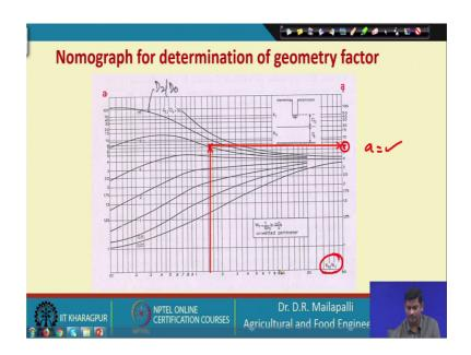
So, just knowing the you know K knowing the K b by K t and D b by D t. So, then you will be finding out the point where it is going to intersect and from there just project on to the y axis right. So, that will give the corresponding a value that will give the corresponding a value here ok. So, this way you can estimate the a values ok.
