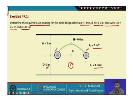
So, in this I mean from the previous lecture using the Hooghoudt equation so, there is an example. So, determine the required drain spacing for the basic design criteria q or say recharge or the drainage discharge which is equal 7 mm per day and H is 0.6 meter. So, that is we are expecting the highest water table at the center of the 2 drains is 0.6 meter and pipe with outer diameter is 0.2 meter and u which is equal to 0.3 meters that is the wetted parameter of perimeter ok.
