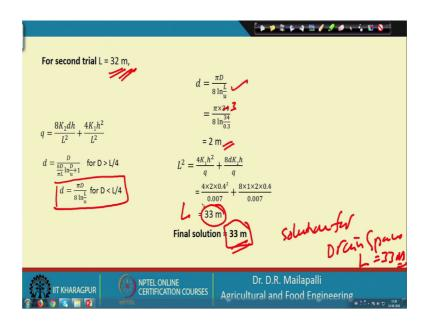
So, let say L is equal to 34 or even 32. So, close to that so, this is the second guess. So, now, L by 4 is that is 8; that means, still it is less than right less than I mean D is less then L by 4 and we are going to use the same equation ok. And this is supposed to be 3 meter and you get 2 meter small d right and then the finally, you get L is equal to 33.
