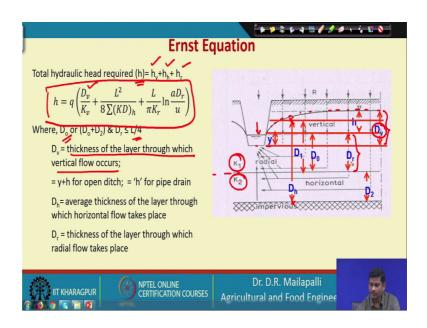
So, in case of Ernst equation, the total hydraulic head required h is equal to vertical, horizontal and radial ok. So, that if you combine all these, you know the vertical,
