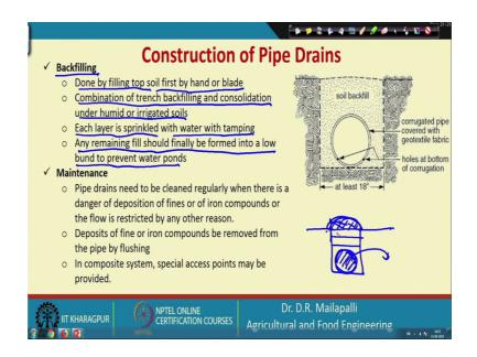
So, the next is construction of pipe drains. So, and then backfilling, this is very important. So, once open the drain and install the pipe to the backfilling needs to be done. So, this is mainly done by filling top soil first by hand or a blade. So, first is the top soil, then the combination of trench backfilling and consolidation, so, then after that backfilling consolidation, so under humid and irrigated soils.
