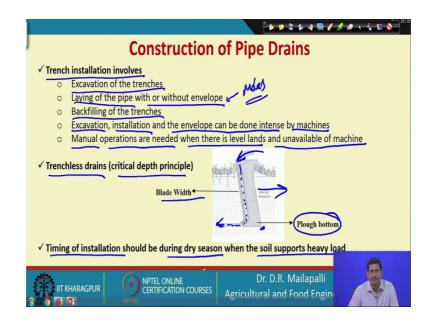
So the next is trench installation, which involves excavation of the trench trenches. The first one is excavation opening the soil and laying of the pipe with or without envelope. So, laying of the pipe with envelope if, the trench is opened without envelope if, the if it is a trenchless ok.
