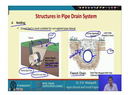
So, this is a surface water inlets. And then the other one is known as the bedding ok. So, the bedding so, the gravel bed is most suitable for corrugated pipe lateral. So, if you see this, so, this is perforated pipe right, you see the holes here. And then water floods the trench then enters the pipe and flow away. So, what happened this is a gravel so right.
