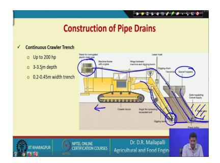
So, the next is the continuous crawler trench, ok. So, this is up to 200 hp and it can make 3 to 3.5 meter deep trenches and 0.2 to 0.45 meter width of trench ok. So, if you see here, so, the continuous crawler trench will have this kind of you know, the crawlers the crawlers. So, then so, this is the corrugated drain pipe ok. So, look at this, the corrugated drain pipe is bounded or to a vertical shaft and then from there this is all the way conveyed to the trench and then it is gets installed.
