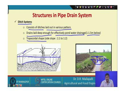
So then there is a ditch system. So, the ditch systems generally, what happens the open ditches. So, if you see in this picture, so, this is the water table right and this is sorry the initial groundwater table. And, if you want to remove water below the root zone here right the open ditch system, so, these are the 2 ditch ditches that will take away the water or drains the water from the root zone. So, the ditch system consists of is laid out in various patterns.
