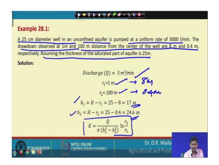
So, the example so, you have a you have a 25 centimetre diameter well in an unconfined aquifer pumped at uniform rate Q is equal to given. So, the drawdown observed at 1 meter and 100 metre distance, are 8 meter and 0.4 meter respectively, assume the thickness of the saturated aquifer is 25 meter.
