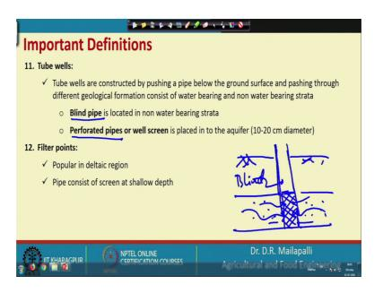
So, here in tube well there are 2 parts; one part one is blind pipe and perforated pipe or well screen. So, this is a pipe if you see ground surface and then there is a aquifer. So, then so this the (Refer Time: 19:26) from top to up to this is called blind pipe, which does not contain any perforation. Otherwise, the next part the below there is a thin pipe. So, which is required because this is the, this is what is that aquifer? So, this collects the water through the perforations.
