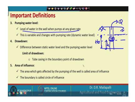
See the pumping water level here so, once you pump water from the well. So, the time at which the water level present in the well is called the pumping water level.
