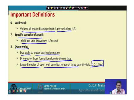
And, then so, next is well yield. So, the well yield is the volume of water discharge from it per unit time. So, in a unit time how much volume of water which is discharged from the well is called well yield.
