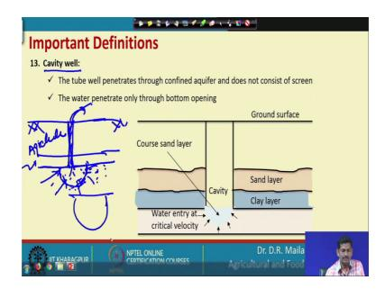
So, then what is the cavity well. So, the cavity well is a tube well. So, opposite to the filter point so, this consists of blind pipe in does not contains any contain any screen pipe. So, here the cavity wells are generally used in clay soils. So, like if you have a clay layer, if you have a clay layer. So, this is a ground surface right and this is a clay layer. So, that is aquiclude right aquiclude.
