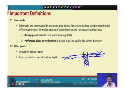
So, water table is shallow you do not require any blind by here. So, directly you can use a screen pipe right the whole screen pipe can be used right. So, because the water table is up here so, all maybe even will be less, but since the water table is shallow you do not require any blind pipe in case of the so, those are filter points.
