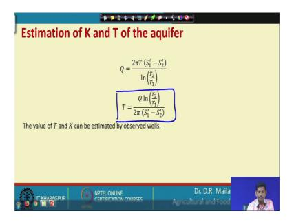
So, this way so, the final so, finally, you get a T is equal to Q into l n r 2 by r 1 2 pi into S 1 dash by S 2 dash. So, let us see an example here.
