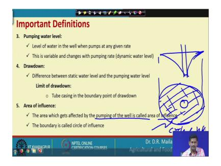
And, area of influence, the area which gets affected by the pumping of well is called area of influence suppose. So, here so, you have a this is a drawdown curve right. So, the area so, the area so, if you take the top loop right. So, this is the well. So, the area which is influenced by this well right is called the pumping of the well is called area of influence. So, this is the area of influence and the boundary is called the circle of influence this is the circle of influence.
