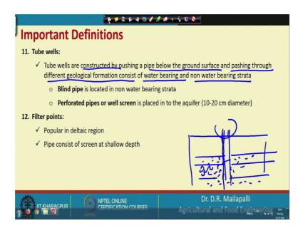
So, then the next is tube wells. So, what is that tube wells? So, tube wells are constructed by pushing a pipe below the ground surface and pushing through the different geological formation, which consists a water bearing and non-water bearing strata. So, this is a tube well is a pipe, which is being pushed down into the into the ground.
