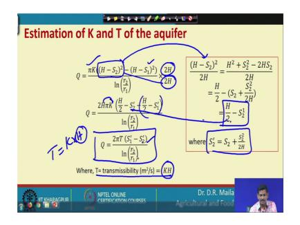
So, the next so, and once that is done. So, the pi K H minus S 2 square, H minus S 1 square into just multiply by 2 H and divide by 2 H. So, take one here and see how it how we can transform. So, H minus H 2 square by 2 H right by 2 H is equal to H square plus H 2 square minus 2 H S 2 by 2 H.
