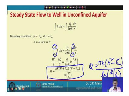
So, put these limits right r w R and if you can integrate this finally, get the equation Q where Q to pi K H plus h w h w into H minus h w. Q is equal to pi k into H square minus h w square divided by l n of R by r w.
