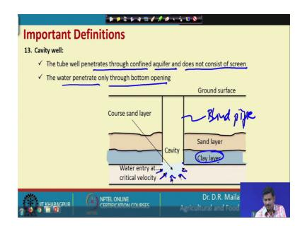
So, cavity well is a tube well penetrates through confined aquifer and does not consist of a screen and the water penetrates only through bottom opening. So, here so, this is a blind pipe and is the ground surface this is a course sand is here and this is clay layer and also sandy layer. So, we are looking for the clay layer. So, once it hits the clay layer and that is it so, water enters the critical velocity just like it clears a bulb here.
