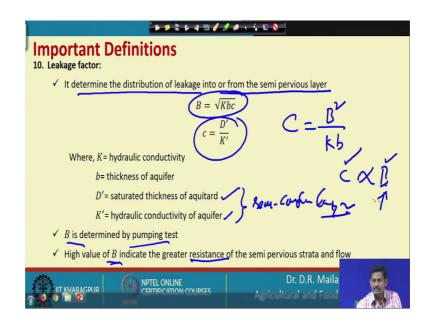
So, and then next property is leakage factor so, in case of leakage factor as I said the determines the distribution of leakage into or from the semi impervious layer. So, are the same equation if we use C is equal to right B square by k b right. So, then B is equal to C k b square root right K b c square root, where c is equal to D dash or b dash by K dash, D dash is saturated thickness of aquifer and K dash is hydraulic conductivity of the aquifer.
