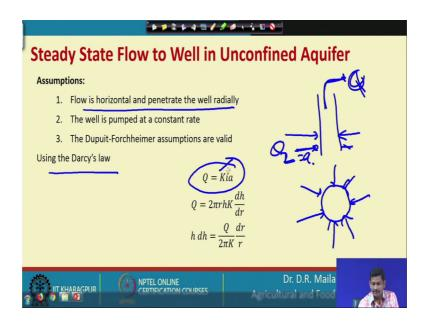
So, here in case of steady state so, there are assumptions that flow is horizontal and penetrating the well radially. So, the flow which is taking place this is horizontal right and also this is horizontal, but radially it is doing it. And, then well is pumped at a constant rate, this Q is constant here right so, then the Q 2, which is also equal to Q 1.
