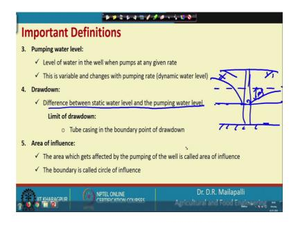
So, then drawdown so, drawdown is difference between static water level and pumping water level. So, the same you see so, this is the bedrock and then have a well. So, static water level and this is the pumping water level right. So, the difference between these 2 will give the sorry so, the difference between these 2 will give the a drawdown. So, that is denoted with S.
