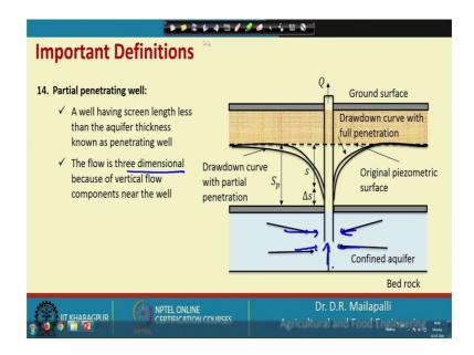
And, the next is partial penetrating well. So, here if you see in previous case, the well was here up to this is a fully penetrating well right. So, in case of partially penetrating well, so the water is flowing through well in 3 dimensional basically.
