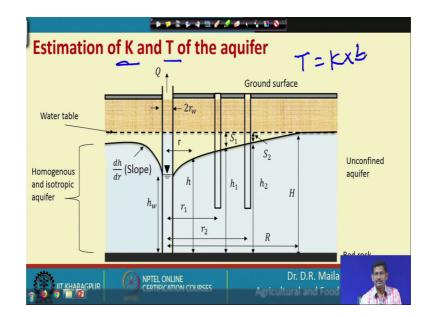
And, in the next so how to estimate the aquifer properties like hydraulic conductivity and transmissivity. So, hydraulic conductivity transmissivity so, K once you have one parameter the other parameter can be estimated because T equal to k into aquifer thickness b. So, here in order to do that so, install a 2 observation wells observation well, one and observation well 2 nearby the pumping well. So, this is a pumping well.
