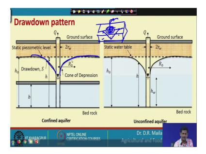
So, this is the pattern the drawdown pattern is like a cone, whereas this is the kind of a cone. So, just like you have you know the spongy material right, this is the spongy material which is initially completely saturated, if you put a straw and take water from here. So, it so, the water which is adjacent to this opening will be first removed, then after that it will be influenced to the extreme points. So, if you see this so, this acts like a cone.
