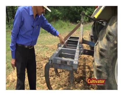
This is another equipment which is secondary tillage equipment. It is a nine end cultivator. You can see that the four tensor in the front, this four tensor are in the front and the five tensor in the back.
