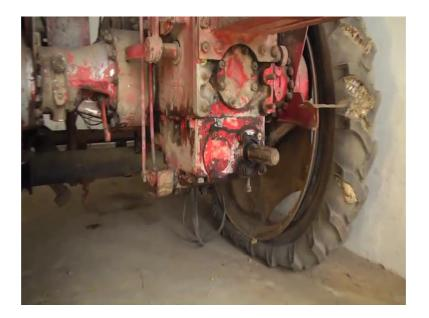
Here, it is a front PTO. Have a look at this same six s plank, but this front PTO and the weight distribution, you can see here that this is a long beamed where the weights are kept and the balance of the weight with respect to the rear weight by giving weights on these.
