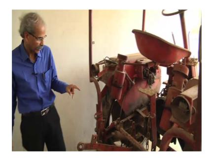
The PTO, the back PTO is over here just like ours, but all the locations of everything was at this position. You can see the exhaust of the other tractor and exhaust over here. Now, the exhausts are located over here in contrast to the new tractors. The difference here is that these tractors we were not taught of particularly with respect to the operator because these were made well in 1940's or so and this is a Russian tractor.
