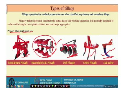
See the types of tillage equipments. Now, you will see that for tillage we need mainly two types of equipments. First is the primary tillage operation where see we require primary tillage, primary tillage implements; Now, a mold board plough, a reversible plough, a disk plough, a chisel plough or a sub soiler.
