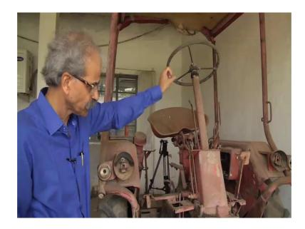
The steering balls; operated through this is a similar kind of operating system of the steering which are here the way we have Ackerman type of a steering system.
