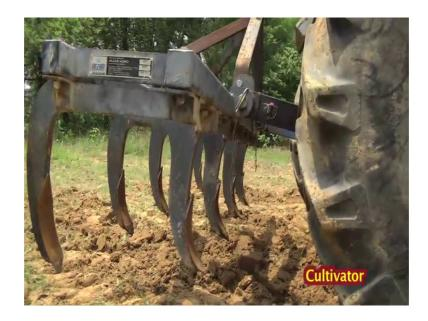
This is the shovel; this is which is called a reversible shovel. Now, there are others which are spring connected, this rigid one and job of this is to break the clots which have been prepared by the mold board plough or the disk plough. Now, the operation of this plough actually preparation of the field will be at least twice operation of this. This will be required for preparing the field as you have seen in the case of a rotavator.
