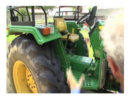
All these are well distributed, its say four wheeled drive tractor. Generally when we have a four wheeled drive tractor, we will have the weight distribution approximately on the front axle and rear axle, approximately 50-50. But when we have a two wheeled drive as we have in other tractors, we have about 65 to 70 percent of the weight on the rear axle and about 30-35 percent weight on the front axle, but this is a four wheeled drive tractor.
