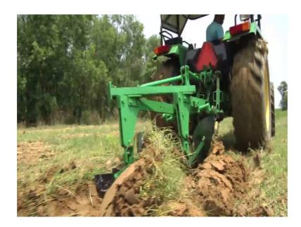
Continuation of what I said earlier, the mold board plough and the disk plough, these are the two primary implements which are used for opening of the soil. When the mold board plough is generally used for first opening of the soil where the land is not that stony or very grassy, but when it is very stony land, there the mold boards are not used. Generally we use these disk ploughs.
