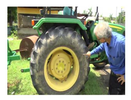
Now, see here it is 16.9 into 28. Now, this 16.9 into 28, this means that 16.9 is the section width which we can call from here or even we can take if draw a scale from here and then, this width is 16.9 which is in inches. Mind you this is very important to be noted that this is in inches, then 28, these also in inches and this talks of the rim width from here to here.
