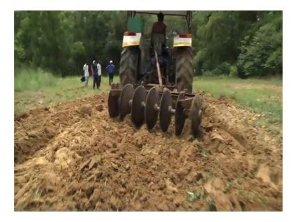
We have seen that two types of implements, particularly the primary tillage implements which are mold board plough and disk plough, there we had seen that the soil, a bigger clots are coming out. Now, when we operate the secondary tillage implement, the aim is that these clots will be smaller and the soil will become very friable. So, you can see that the soil become friable as case of say the big clots which are coming. So, the aim is to
