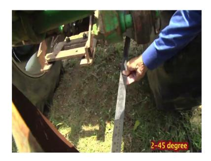
If you take the disk, this is the angle which we maintain is the disk angle which is here. Now, this disk angle and umm tilt angle, both angles are very important. The tilt angle generally varies between about 15 to 25 degrees or so and the disk angle varies between 42 to 45 degrees with respect to the line of travel. These are very important when we want the total output of these disks.
