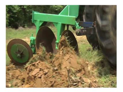
As you can see that the disk has thrown, it scooped the soil onto one side from here, you can see this and the next one which will come here, again it will put on the same scoop soil. So, this is the way it throws the soil here. The inversion is not to the extent that you get there, but only because of the disk this implement.
