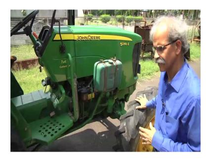
We can see here, right from here is our radiator and then, the engine, the transmission, then differential and final drive.
