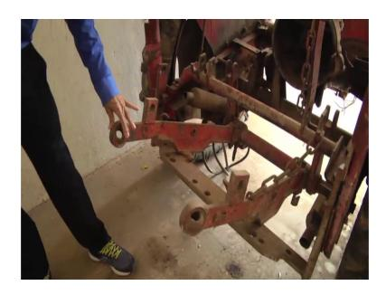
This is the one link which has the point here, this another link which has the point here. Here there is no top link.
