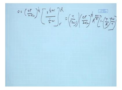
Now if we go to that, yeah this we had developed that velocity was at any instance v was delta p, right? By 2kL, right? To the power 1 by n, right? And r to the power 1 by n plus 1 divided by 1 by n plus 1 within that limit of r to R and this was n by n plus 1, right? Into delta p by 2kL to the power 1 by n and R to the power n plus 1 by n into 1 minus r by R to the power n plus 1 by n, right? This we had developed in the previous class, right?
