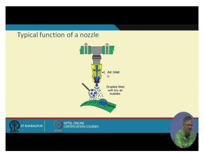
Typical flow throw through nozzle like this this diagram we had shown this is another typical function of nozzle where air is going in and you see that many nozzles are used particularly in spray drying if you see that spray dryer where it is there. So nozzles are there which are atomizing the inlet of the fluid and they are also similar behaviors you can expect, right?
