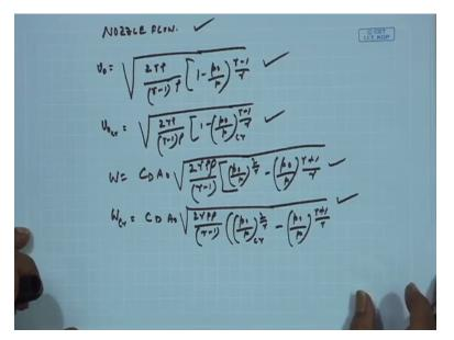
So if we go back to that previous which we have already written here that in the nozzle flow the velocity is like this and velocity under critical condition is like this discharge was like this and discharge under critical condition was like this. Now what was that critical condition?
