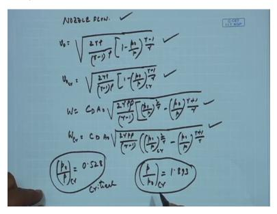
If we just remember a little that we said if the ratio of p0 over p if this is equal to 0.528, then we call that this is under critical pressure ratio, right? Or the converse is also true that if the pressure ratio of p by p0 is equals to 1.893, then also it is under critical pressure ratio that is called p0 by p under critical this is also p by p0 under critical, right? So if we apply that, right?
