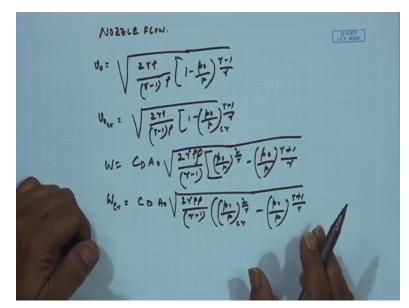
Now that if you remember we had given that v0 was equals to v0 was equals to, yeah under root 2 gamma p divided by gamma minus 1 into rho into 1 minus p0 by p to the power gamma minus 1 by gamma, right? This was our normal velocity and velocity under maximum which we call it to be critical velocity and this was under 2 gamma p, right? By gamma minus 1 into rho into 1 minus p0 by p to the power gamma minus 1 by gamma under critical, right?
