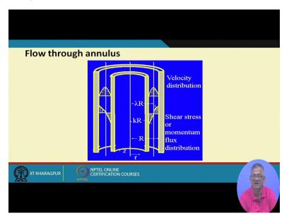
So in any case let us take one such here you see we have neatly drawn that this is the one pipe and this is a another this is the section of the pipe which is having annular flow, right?
