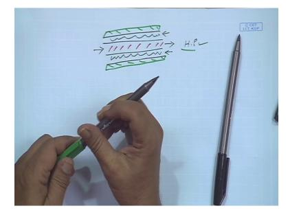
If a fluid is flowing through that we have found out and with that Hagen–Poiseuille's equations we developed, right? Now, if the situation is like that in many cases you will see you have a double tube heat exchanger, right? So you have a double tube heat exchanger one fluid is flowing through this so that you can find out with this Hagen–Poiseuille.
