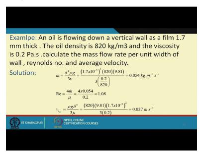
An oil is flowing down a vertical wall as a film 1.7 millimeter thick the oil density is 820 kg per meter cube and the viscosity is 0.2 Pascal seconds. Calculate the mass flow rate per unit width of wall Reynolds number and average velocity. So this is a then pure case of falling film where we are saying that an oil is flowing down a vertical wall as a film 1.7 millimeter thick, so thickness of the film is also given,
