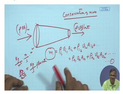
So here that is what we are saying, now if we tell to be total mass aim so that is equals to say at different points rho 1 into velocity at that point in at the inlet v1 into area of the inlet at that point Ai1 plus similarly rho i this is at the point 2 v at the point 2 and area at the point 2.
