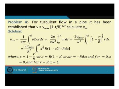
for a turbulent flow in a pipe it has been established that v is equal to v max into 1 minus r by R to the power 1 by 7, so then you have to calculate the average velocity.
