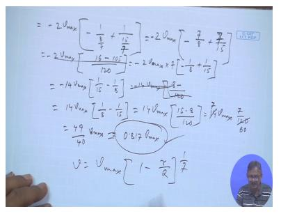
Whereas we started with that relation was v is equals to v max into 1 minus r over R to the power 1 by 7, right? So any such relation if we have, then you can get the average velocity in terms of maximum velocity.
