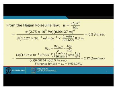
$\mathcal{L} = \frac{\pi \Delta R R^{4} T}{8 R^{4}} = \frac{\pi \left(2.7 s \times 10^{5} l_{R}\right) \left(0.00127\right)^{4}}{8 \left(1.127 \times 10^{5} \frac{m^{4}}{m} \times \frac{1}{100}\right) 0.5 m}$ = 0.5 Pa. Sec Ner = Dozant =  $= \underbrace{(1)}_{x} \underbrace{(1)}_{x} \underbrace{(1)}_{y} \underbrace{(1)}_$
