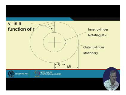
So here the same problem if an incompressible fluid is flowing between 2 vertical coaxial cylinders, and the inner one is rotating with than angular velocity omega, determine the velocity for the tangential laminar flow, right? Now the inner one is rotating and the outer one is fixed, so this outer cylinder is stationary and inner one is fixed rotating rather with an angular velocity of omega, right?
