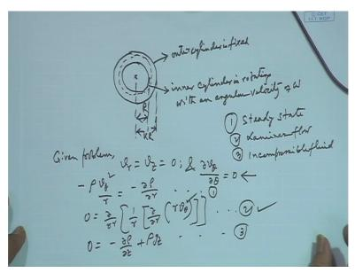
And kept that R and KR as the 1<sup>st</sup> case that this is R and this is kR, right. If you keep them like that then we can say that the problem can be defined like this, we have one inner cylinder, we have one outer cylinder this is the center, right. This outer cylinder is fixed and the inner cylinder is rotating with an angular velocity of omega, right. And we get as earlier the same, this is R and this is KR that is K is multiple more than one, right. So that KR is
