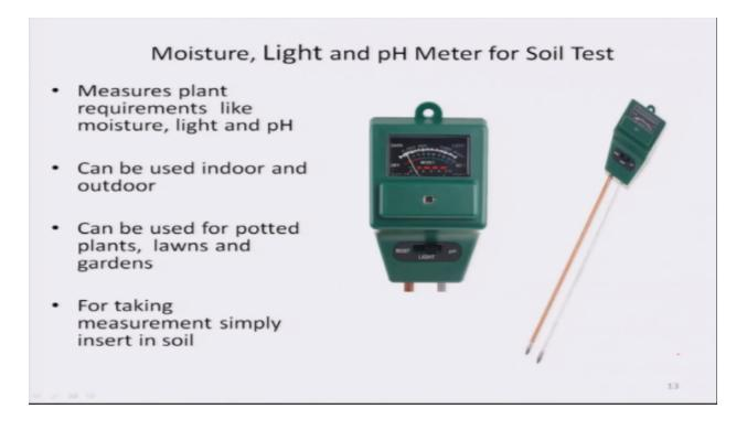
To see how sensors are helping in collecting information about various plants and soil related parameters we are going to see the functioning of a very simple moisture light and pH meter for soil test. The speeder measures plant requirements like moisture, light, and pH. It can be used indoor and outdoor. It can be used for potted plants, lawns and gardens and for taking measurement it is simply inserted in soil.
