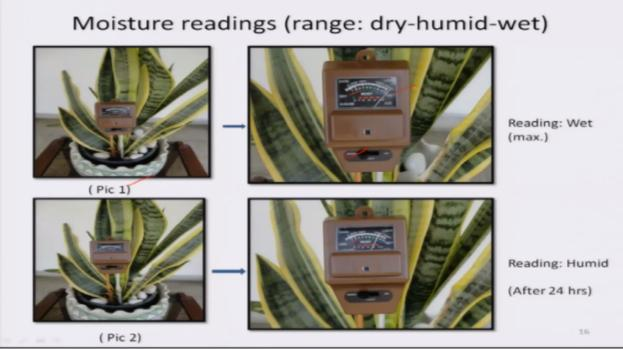
For moisture reading switch is set to moist position. In picture one needle is showing maximum reading when the reading was taken after one day. The moisture content had decreased and the needle had moved back as you can notice in picture 2.
