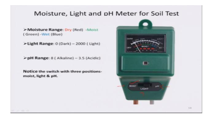
The meter has a switch with three settings; for moisture, light, and pH. When the switch is on moist the needle gives reading for moisture level. When it is on light it gives reading for the light intensity. When it is on pH it tells pH level. As you can notice moisture range is from dry to moist to wet. Light ranges from 0 to 2000 and pH range is from 8 to 3.5.
