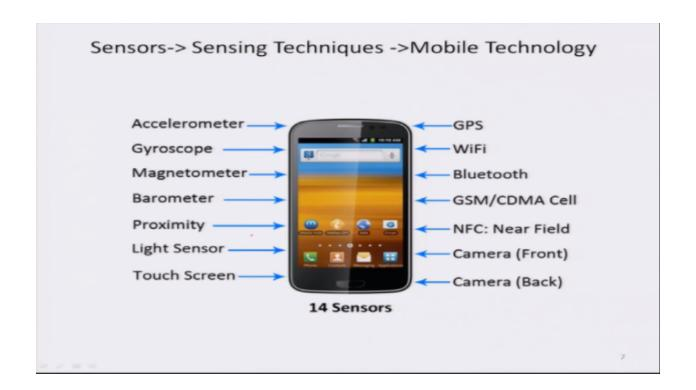
Mobile technology uses many sensing techniques and a smartphone is generally equipped with proximity range sensor, touch sensor, tilt sensor, and as you can notice that there are 14 sensors in this picture.
